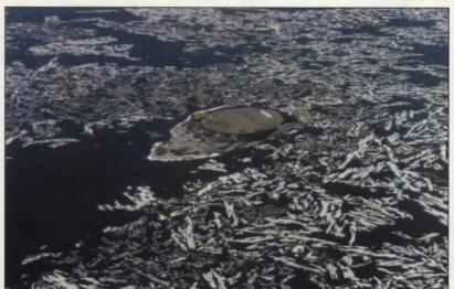
Figure 8 - 29 The ice-free, lee-side of an artificial island in dynamic, broken ice where the mechanical recovery of oil may be possible
