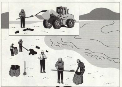
Figure 5 - 34 Manual removal; inset illustrates shoveling oiled material directly into front-end loader to reduce a transfer step
