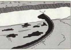
Figure 5 - 18 Shore-seal boom
