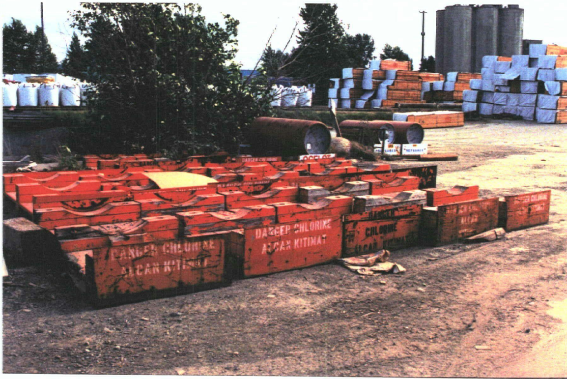
Chlorine tanks saddled in cradles on Rivtow lot Note: The road way on either side of tanks without any containment.
