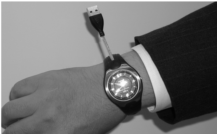
Data storage devices can be disguised as common objects. This USB data watch and pocket knife left have a capacity of up to 256 megabytes and 1 gigabyte respectively.
