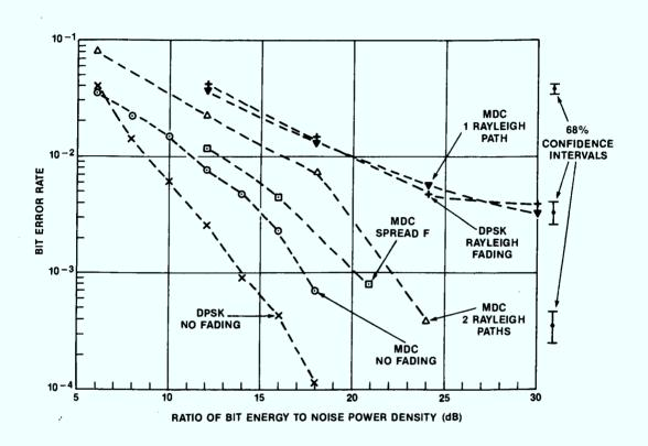
Figure 3.9 Simulation results for CCIR noise.
