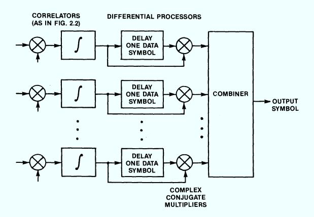
Figure 2.4 Differential demodulation and combining.
