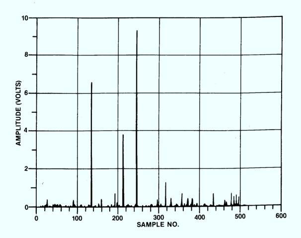
Figure 3.6 Sample of CCIR noise —  $V_d = 20.5 dB$ , 1 volt rms.
