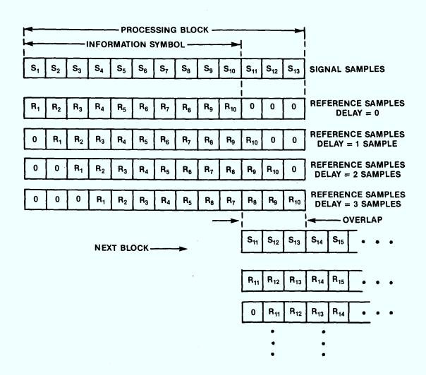
Figure 2.3 Illustration of multiple-delay correlator block processing timing.
