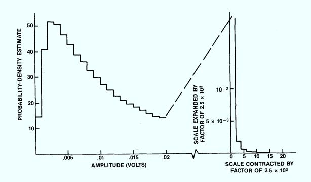
Figure 3.7 Histogram of CCIR noise amplitude —  $V_d=20.5dB$ .
