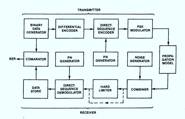
Figure 3.1 Simulation experiment setup.
