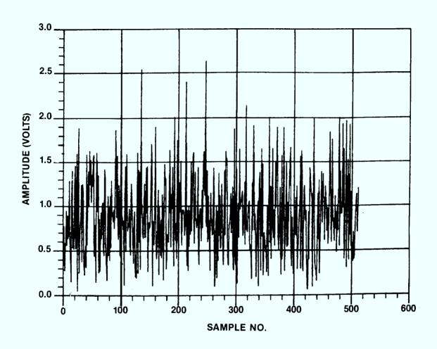
Figure 3.4 Sample of Gaussian noise (Rayleigh amplitude  $-V_d = 1.05 dB$ ).
