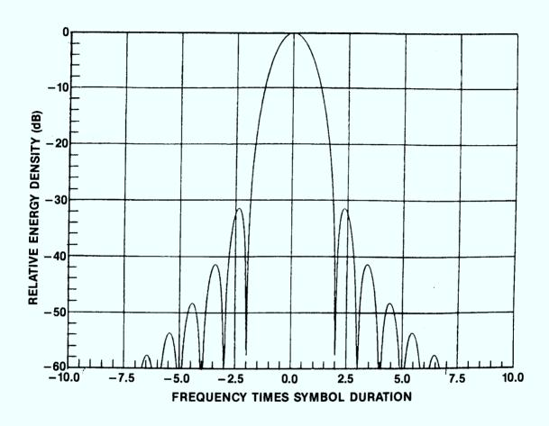
Figure 3.2 Spectrum of Hanning-shaped element.
