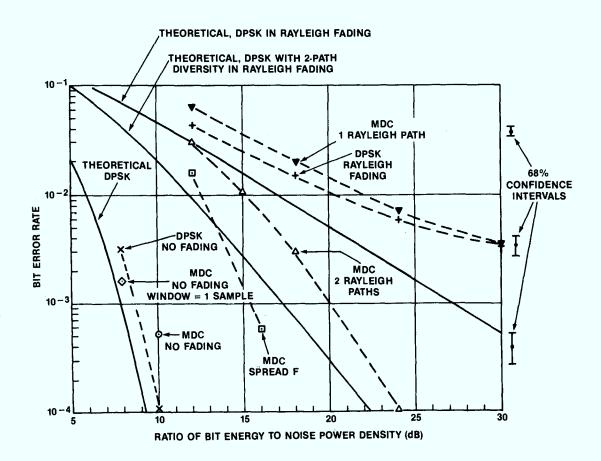
Figure 3.8 Simulation results for Gaussian noise.  $MDC = multiple\text{-}delay \ correlator.$
