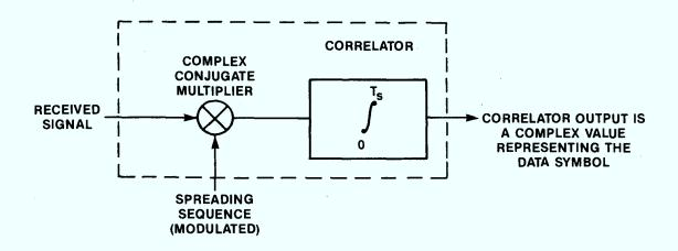
Figure 2.1 Direct-sequence demodulation using a correlator.
