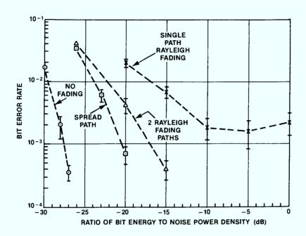
Figure 3.10 Simulation results for multiple-delay correlator in CCIR noise and limiting. 68% confidence intervals shown.
