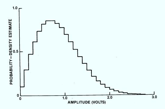
Figure 3.5 Histogram of Rayleigh noise amplitude —  $10^6$  samples.
