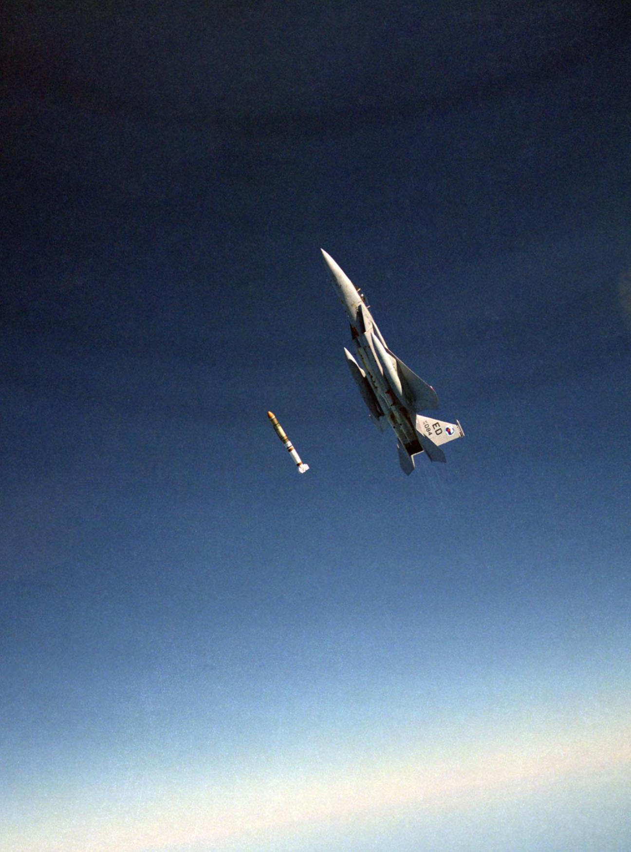
An air-to-air left side view of an F-15 Eagle aircraft releasing an antisatellite missile during a test.
