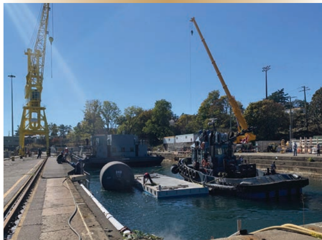
Figure 3. The Esquimalt Harbour tug CFAV Tillicum (YTM-555) prepares to pull the second of two USN submarine camel fender barges out of FMF drydock for return to service at the end of the second docking work period on Aug. 31. In the background is a large YOM-250 environmental barge that was docked with the camels.
