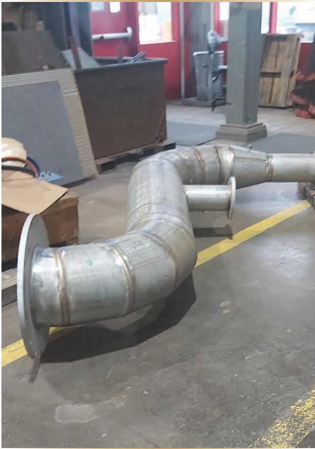
Figure 7. A portion of the new engine intake and exhaust fabricated by Fleet Maintenance Facility Cape Scott.
