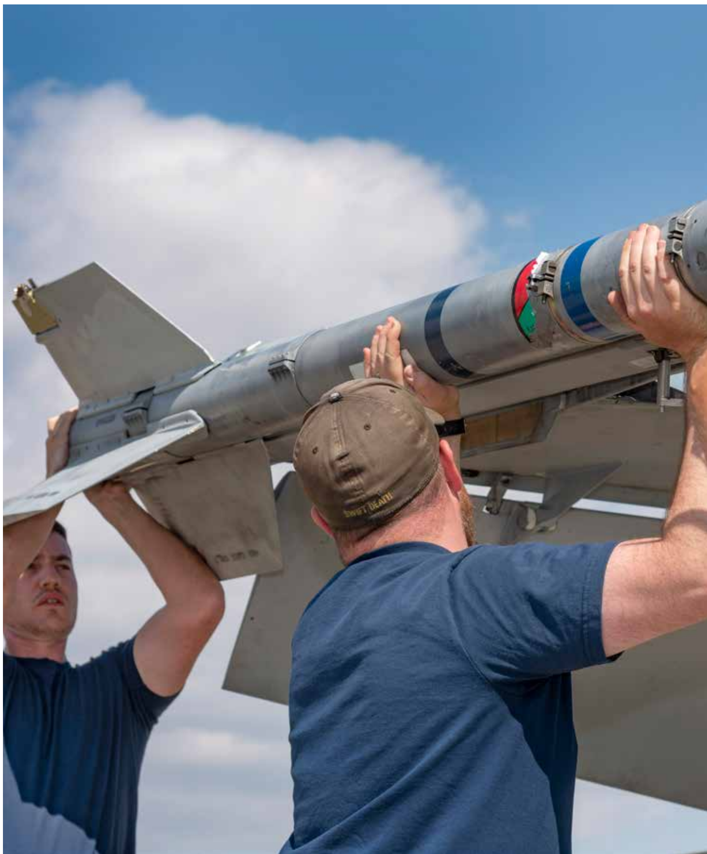
Air Weapons Systems Technicians from 401 Tactical Fighter Squadron load an AIM-9 Captive Air Training Missile (CATM) on a Royal Canadian Air Force CF-188 Hornet during Operation REASSURANCE–Air Task Force Romania at the Mihail Kogălniceanu Air Base, Romania on September 5, 2019.
