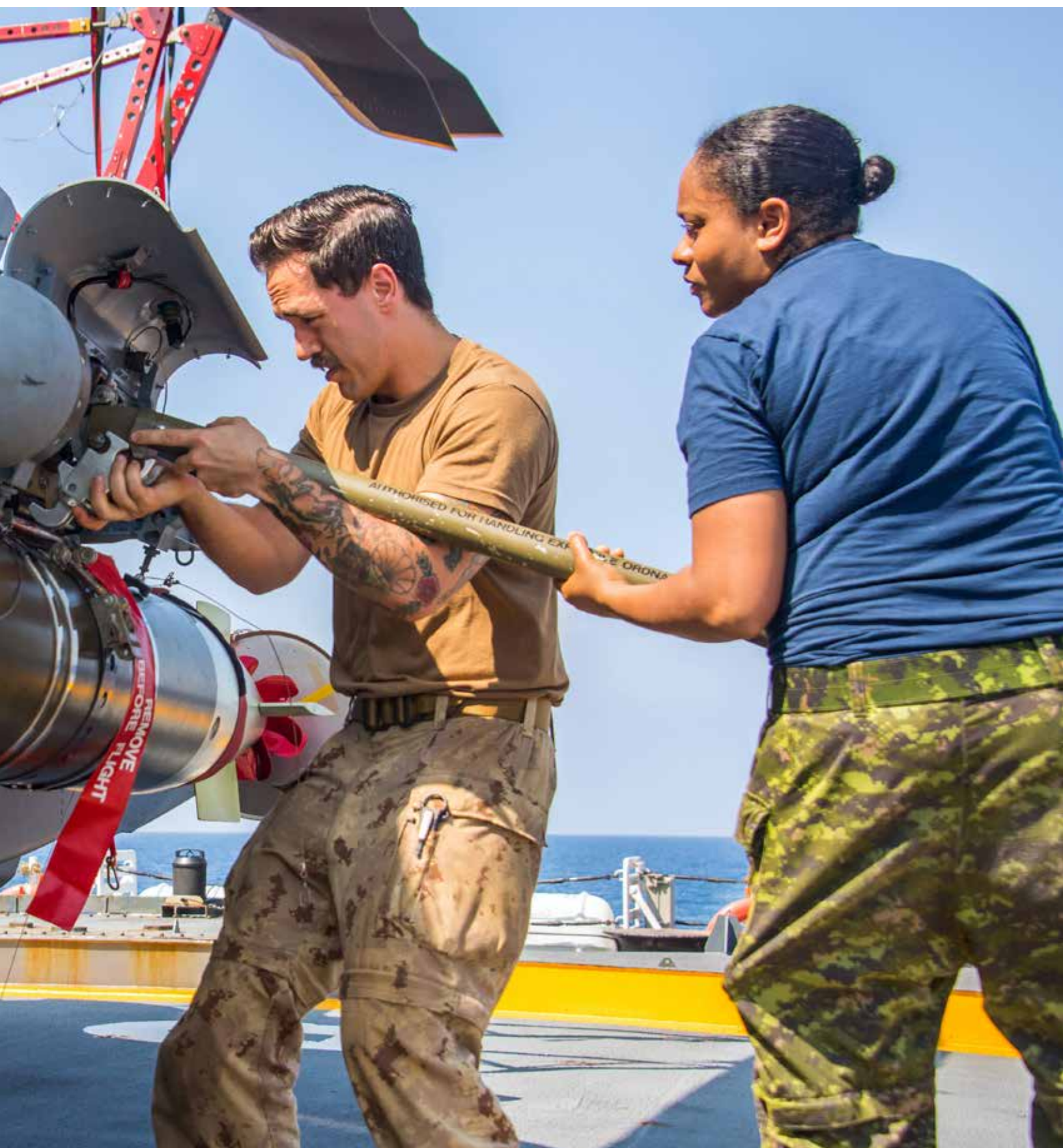
Members of HMCS REGINA's Air Detachment, Master Corporal Jonathan Audet (left) and Corporal Shannon Clayton (right), mount a torpedo on to Bronco, the CH-148 Cyclone helicopter during Operation ARTEMIS, in the Pacific Ocean on April 7, 2019.
