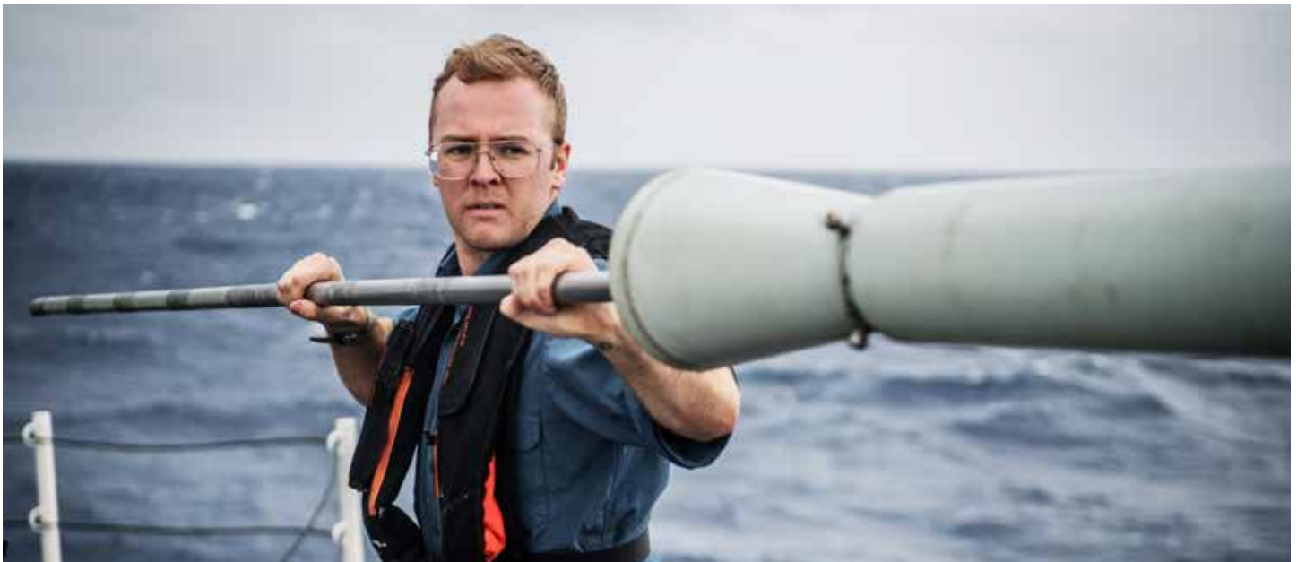
Weapons Engineering Technician, Able Seaman Elliot Poole cleans the barrel of the .57-millimeter gun as part of pre-fire maintenance on board HMCS OTTAWA while deployed on Operations PROJECTION and NEON on October 17, 2019.
