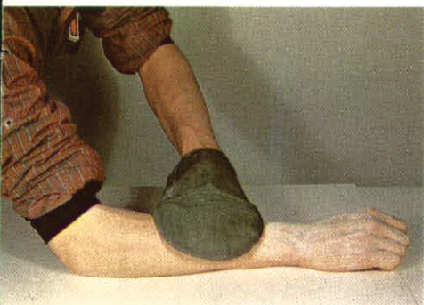
A DREO team developed this porous mitt for dispensing Fuller's earth to decontaminate skin which has been exposed to a liquid chemical agent.
