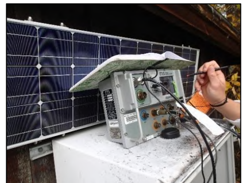
Figure 3. Real time water temperature logger installation on Stuart River.
