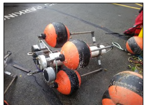
Figure 2. Acoustic mooring before deployment.
