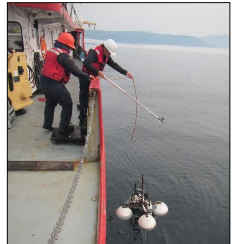
Figure 2. Mooring being recovered from the Vector.
