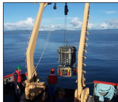
Figure 2. Deployment of a rosette, a deep water sampling apparatus.
