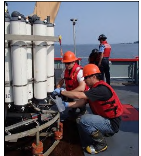
Image 1. Sea water extraction from an instrument profiler that measures water quality.
