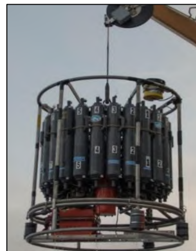
Image 2. Deployment of a rosette, a deep water sampling apparatus.
