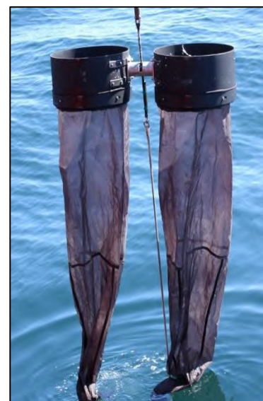
Image 1. "Bongo" nets used to sample the zooplankton.
