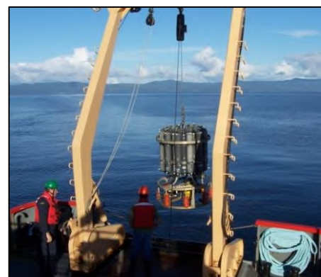
Image 1. Deployment of a rosette, a deep water sampling apparatus.
