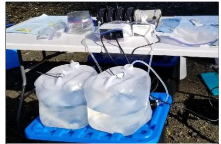
Image 1. Field set-up to filter environmental DNA sample.
