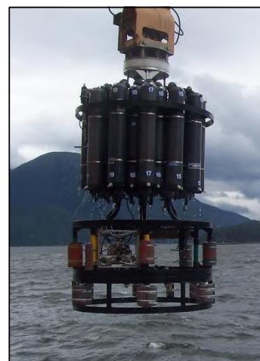
Image 1. Deployment of a rosette, a deep water sampling apparatus.
