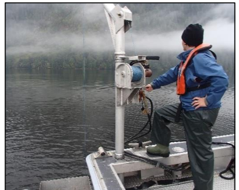
Image 1. Deploying a Van Veen Grab for benthic sampling.
