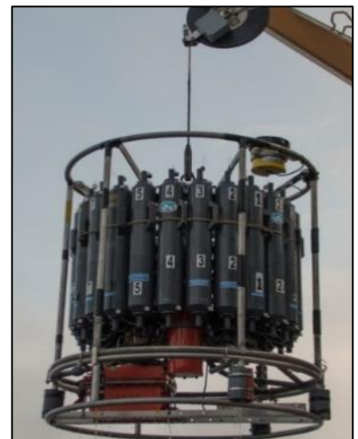
Image 2. Deployment of a rosette, a deep water sampling apparatus.
