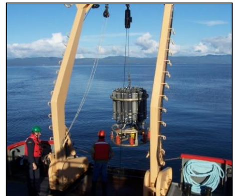
Image 1. Deployment of a rosette, a deep water sampling apparatus.
