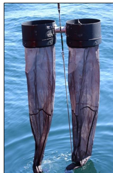
Image 1. "Bongo" nets used to sample the zooplankton.
