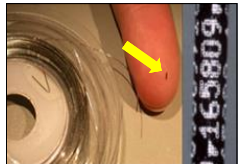
Image 2. Individual tags are cut from a spool of wire and are 1.1 mm long.
