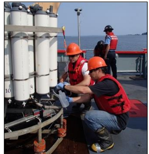
Image 1. Sea water extraction from an instrument profiler that measures water quality.
