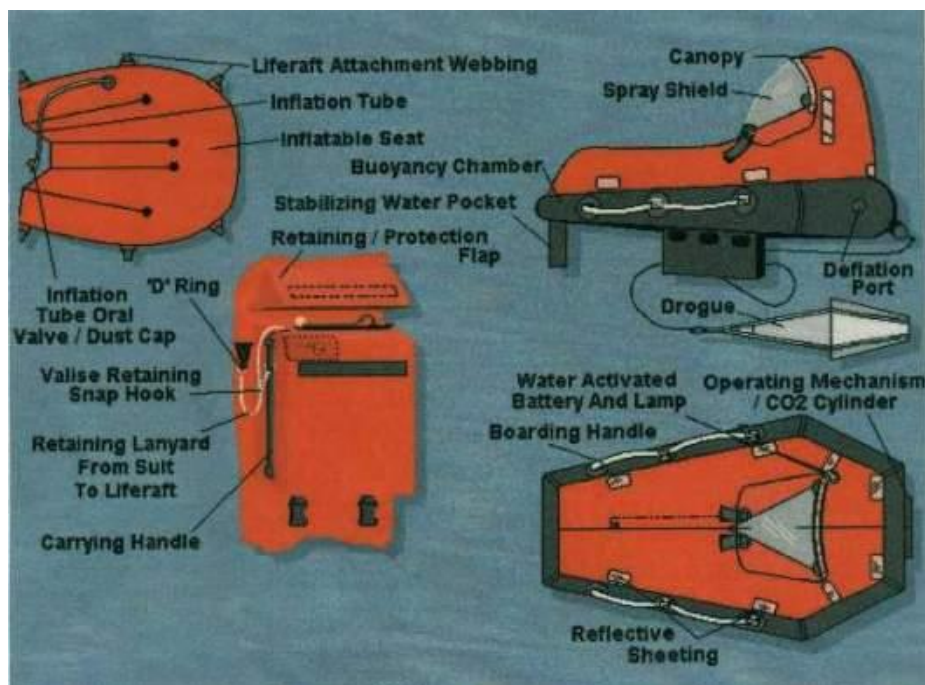
Mk 18 One Man Life Raft which comes with Submarine Escape Suit
