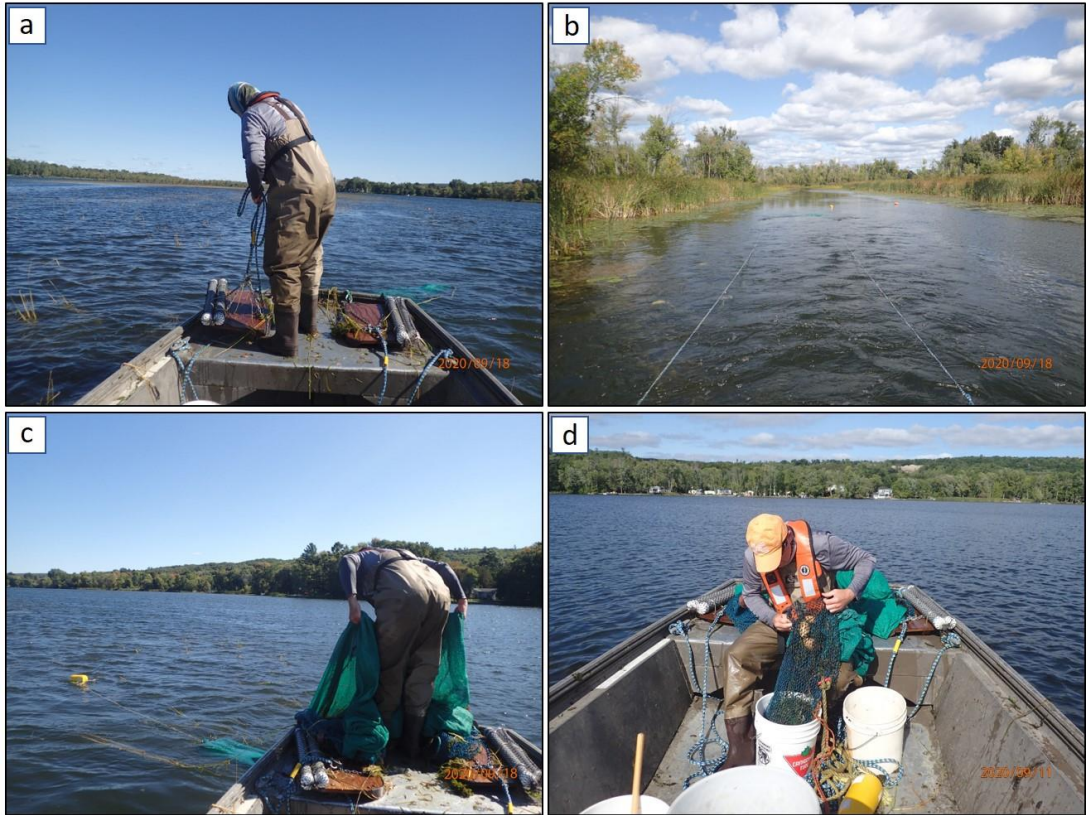
Figure 2. Photographs showing the Mamou trawl during operation: a) lifting the floating doors that open the net, b) towing the trawl, c) retrieving the trawl, and d) emptying the cod.
