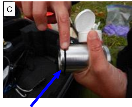
Figure 2.1. OSMOS eDNA backpack sampler filter housing parts.
