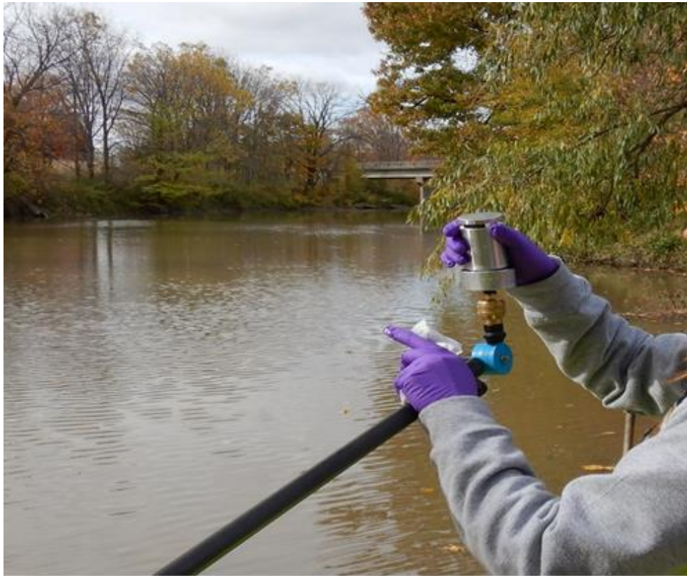
Figure 2.5. Collecting filtered samples and replacing filtered samples Keeping the filter housing inverted pivot the pole towards the shore to change the filter.
