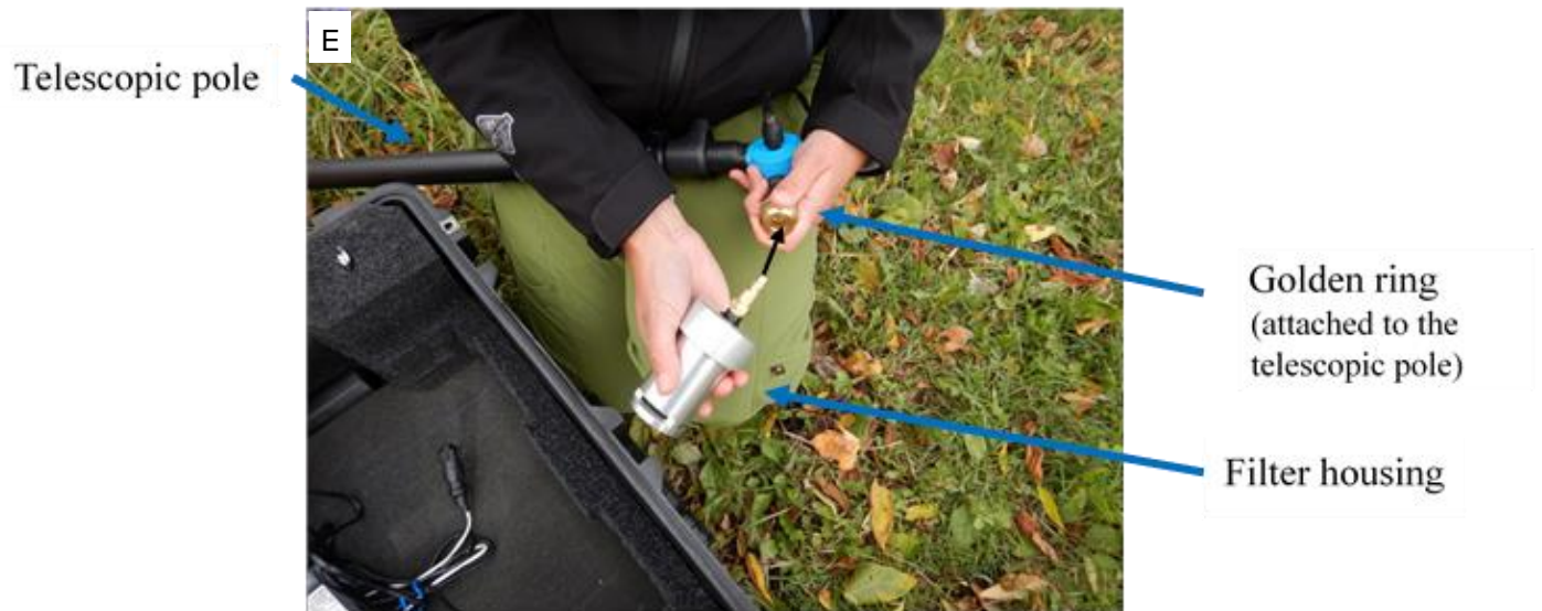
Figure 2.2. (continued). OSMOS eDNA backpack sampler parts and assemblage. The length of the telescopic pole can be adjusted (D). The filter housing is attached to the end of the telescopic pole (E).
