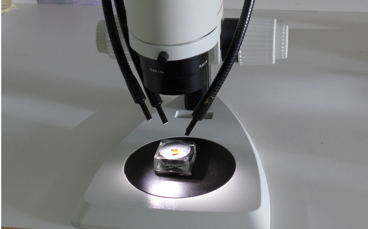
Figure 18. After orienting the burnt otolith in the plasticine, the gooseneck fibre optic lights are bent into position and angled to best illuminate the growth pattern for counting.
