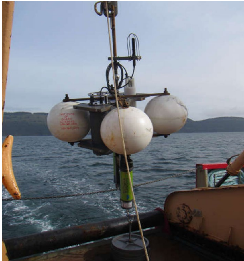
Figure 2: One of the PAM moorings being deployed. Each mooring is equipped with four white floatation spheres to keep the moorings vertical on the sea floor and equipped with a dual set of acoustic releases for redundancy during recovery and held down by a 100 kg anchor. The hydrophone is positioned 2 m above the sea floor.
