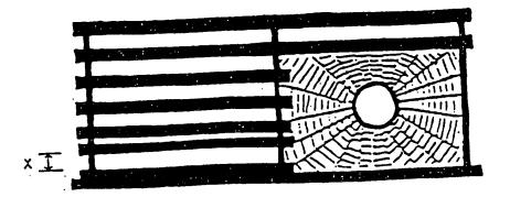
Figure 4 - Diagram of a lobster trap used in the Salmon Beach or Miminegash study where the wooden lath space, X, is varied to 34.9, 37.1, 38.1 or 44.4 mm.
