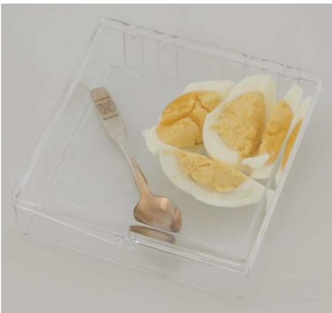
Figure 1a: A transparent box containing a silver-plated spoon and a hard-boiled egg: initial exposure.
