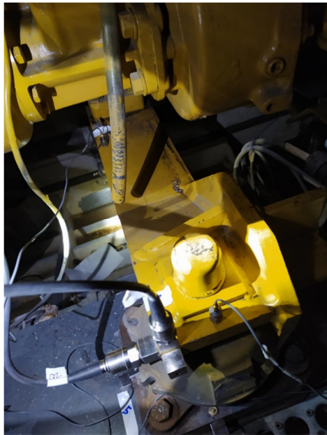
Figure B.5: Hammer test locations—port propulsion diesel foundation.
