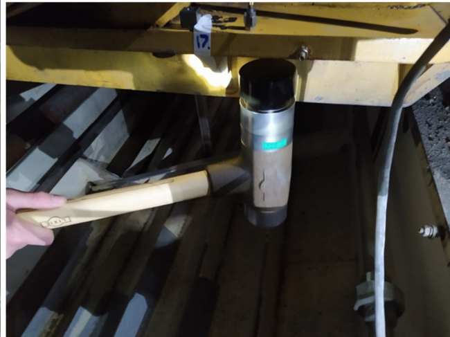
Figure B.5: Hammer test locations—port propulsion diesel foundation.
