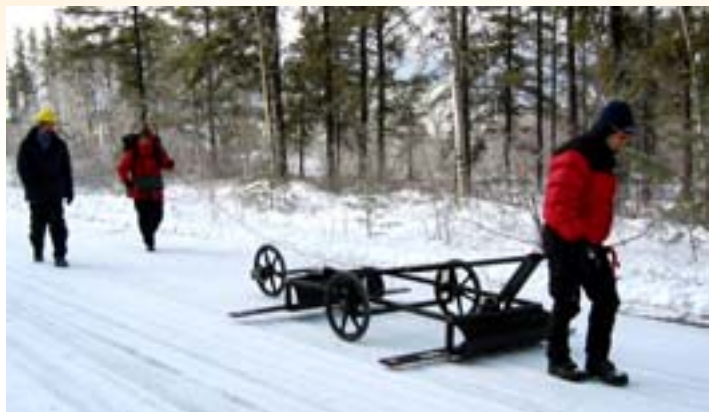
PulseEKKO 100 with its kart and Odometer used on the Abitibi esker project, November 2004
