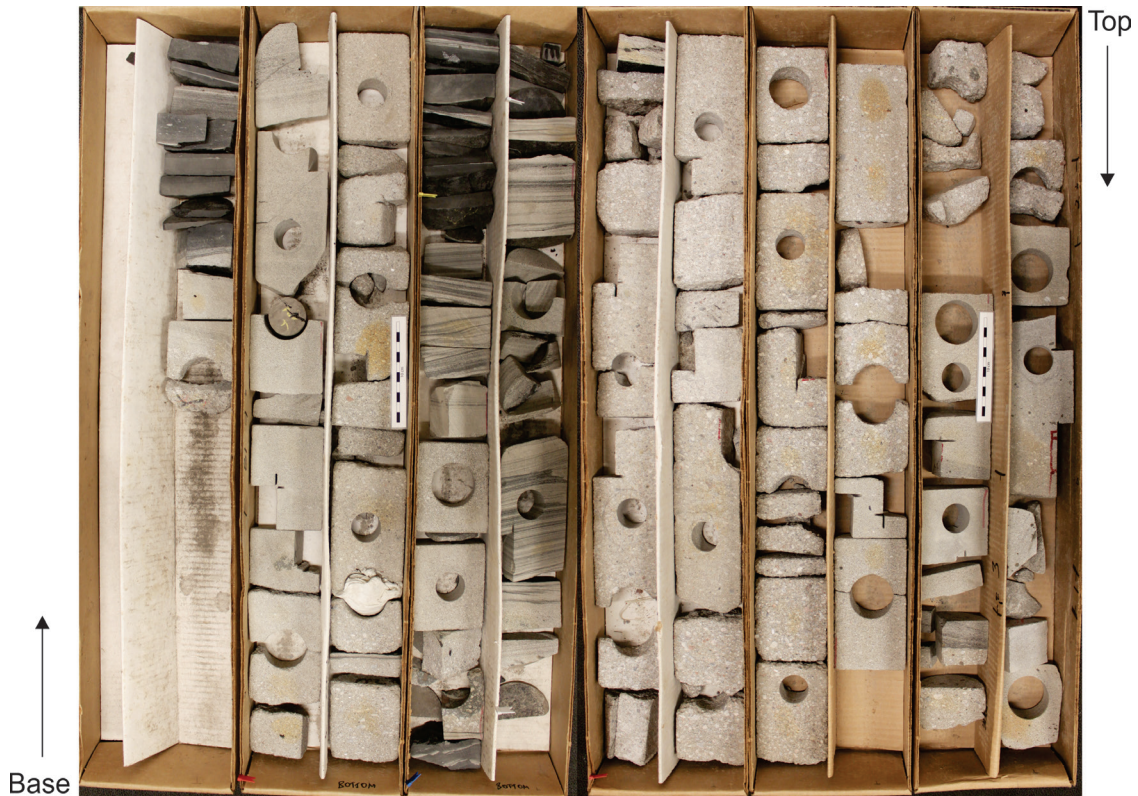
Figure 33. Photographs of core 1, Herjolf M-92, showing the two major facies of blocky, pebbly sandstone (much of the core) and interbedded sandstone and shale (two intervals in the lower part of the core). Scale bar = 10 cm. NRCan photo 2019-369, 2019-370. Both photographs by L.T. Dafoe.
