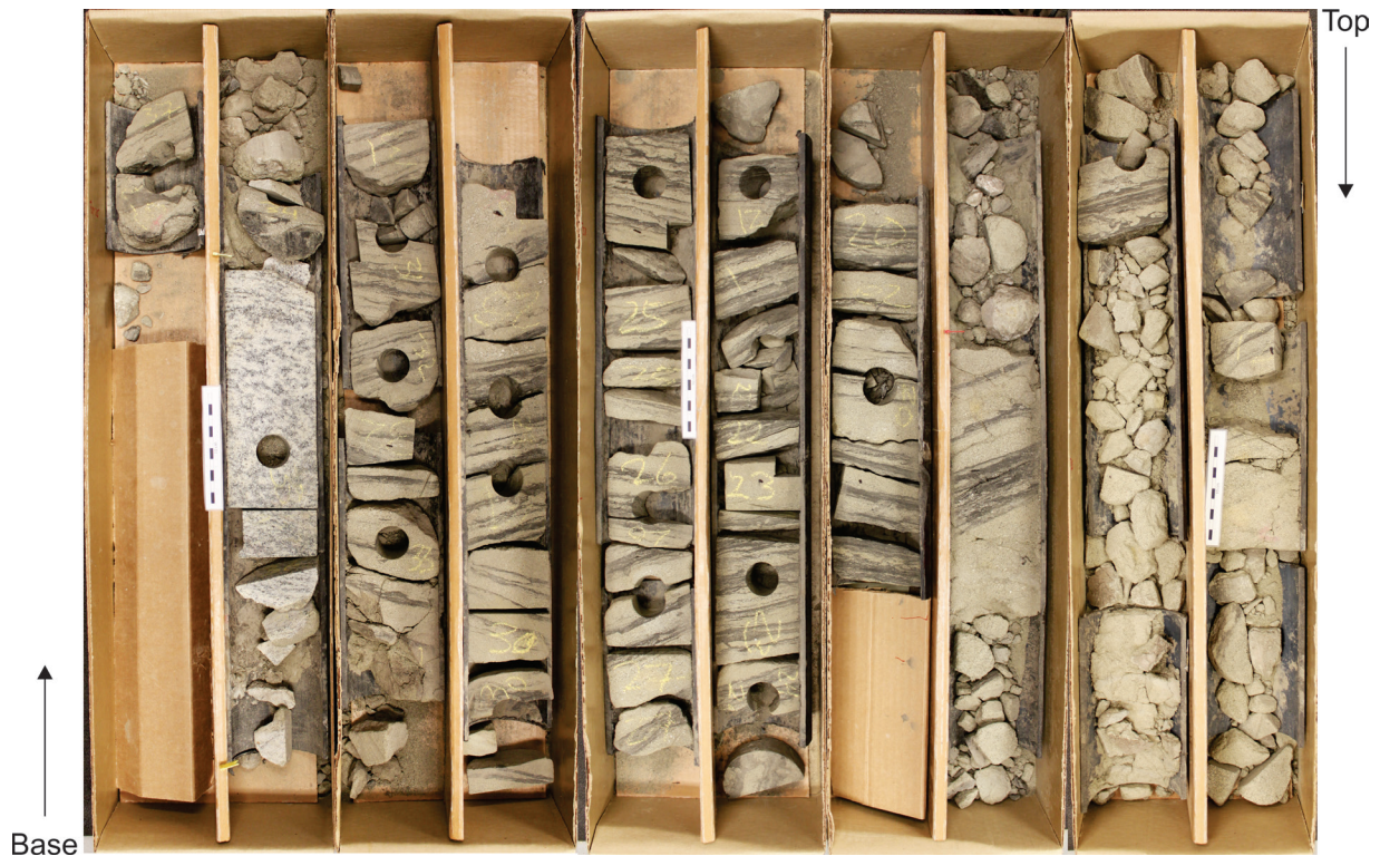
Figure 57. Photographs of core 2, Ogmund E-72 showing the cemented zone near the base and a rubbly section near the top of the core. Scale bars = 10 cm. NRCan photo 2019-439, 2019-440, 2019-441. All photographs by L.T. Dafeo.
