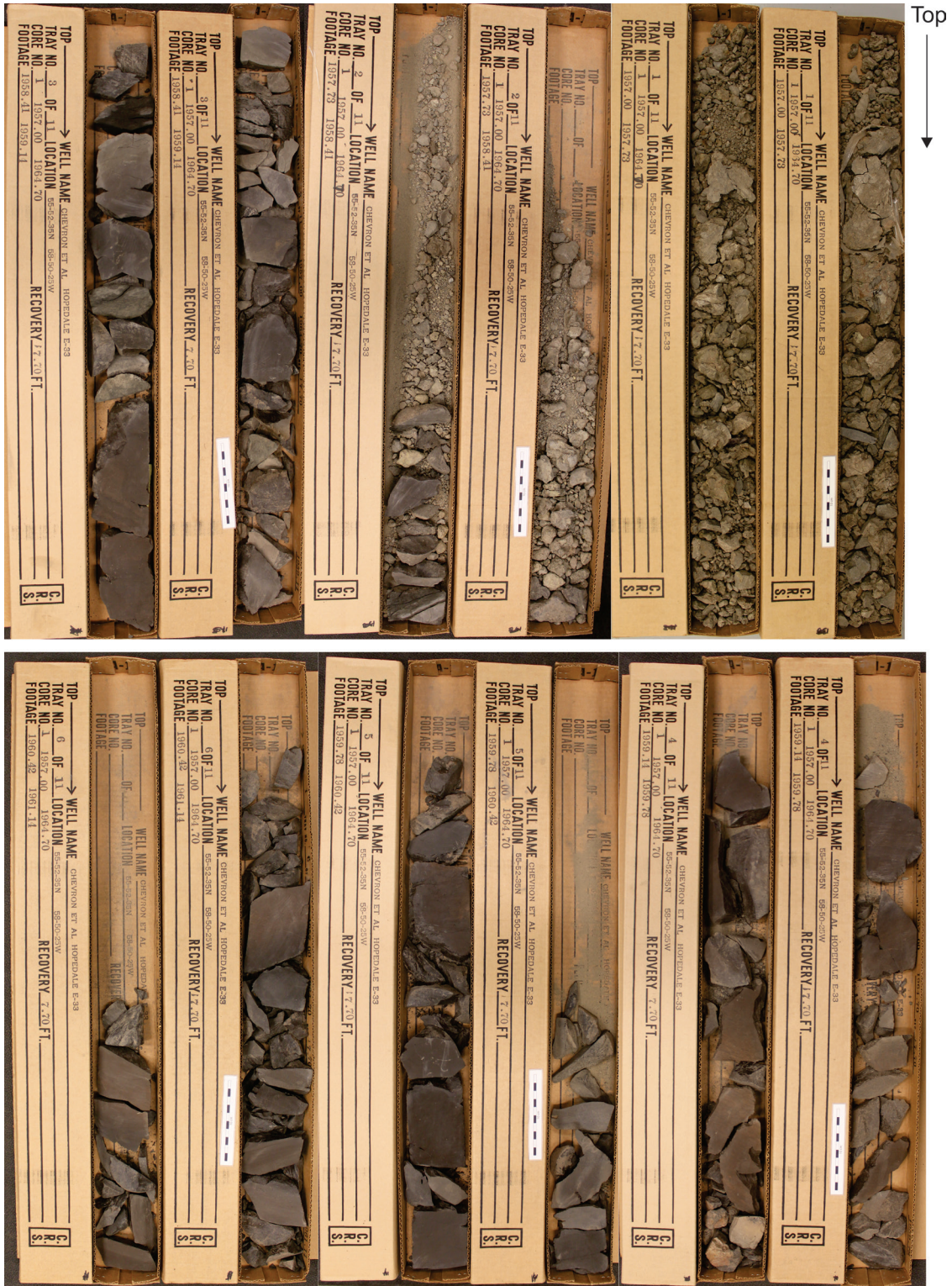
Figure 41. Photographs of core 1, Hopedale E-33. There are two boxes for every interval intended to represent the opposing slabs of the core. Scale bar = 10 cm. NRCan photo 2019-388, 2019-389, 2019-390, 2019-391, 2019-392, 2019-393, 2019-394, 2019-395, 2019-396, 2019-397, 2019-398. All photographs by L.T. Dafoe.
