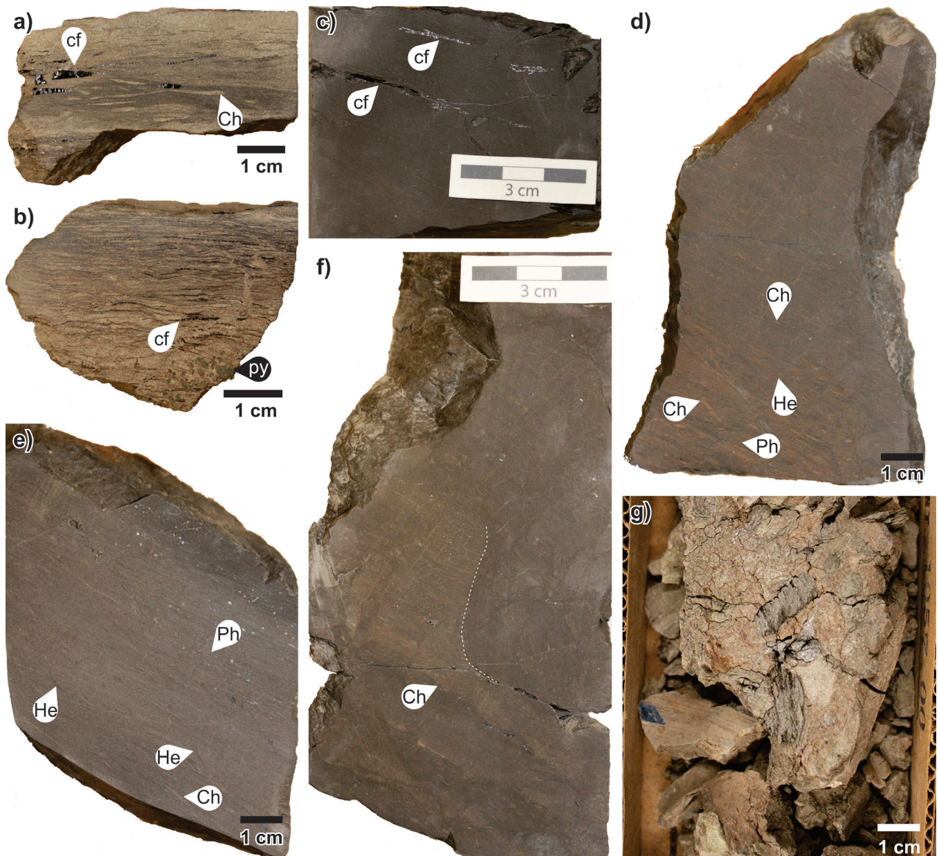
Figure 42. Photographs of core 1, Hopedale E-33. a) Buff sandstone facies, with mudstone laminae, Chondrites (Ch), and coal fragments (cf). NRCan photo 2019-399. b) Sandstone facies with distinct heterolithic composition, coal fragments (cf) and pyrite (py). NRCan photo 2019-400. c) Massive dark grey shale facies with coal fragments (cf). NRCan photo 2019-401. d) Sideritized interval within the shale facies with thorough bioturbation by Chondrites (Ch), Helminthopsis (He), and Phycosiphon (Ph). NRCan photo 2019-402. e) Siltier mudstone interval with intense bioturbation, including Helminthopsis (He), Chondrites (Ch), and Phycosiphon (Ph). NRCan photo 2019-403. f) Mudstone interval with a possible gutter cast structure outlined by the white dotted line, as well as Chondrites (Ch). NRCan photo 2019-404. g) Uppermost part of the core that appears to consist of fragments of bedrock within drilling mud. NRCan photo 2019-405. All photographs by L.T. Dafoe.
