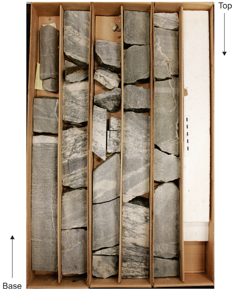
Figure 82. Photograph of core 7, Skolp E-07, showing the Precambrian gneissic basement rock and variation in banding. NRCan photo 2019-495. Photograph by L.T. Dafoe.
