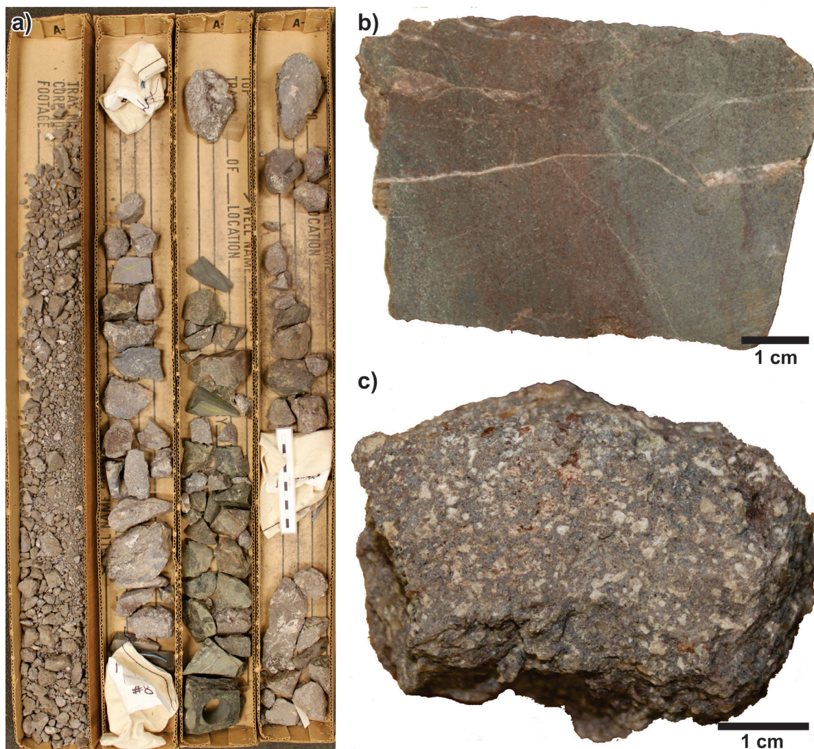
Figure 8. Photographs of core 3, Bjarni H-81. a) Core box sleeves with red-brown to olive green basalt, showing the rubby and weathered nature of the core (scale bar = 10 cm). NRCan photo 2019-302. b) Close-up of fine-grained, fractured basalt. NRCan photo 2019-303. c) Weathered amygdaloidal basalt with white to pink zeolite mineral infills. NRCan photo 2019-304. All photographs by L.T. Dafoe.
