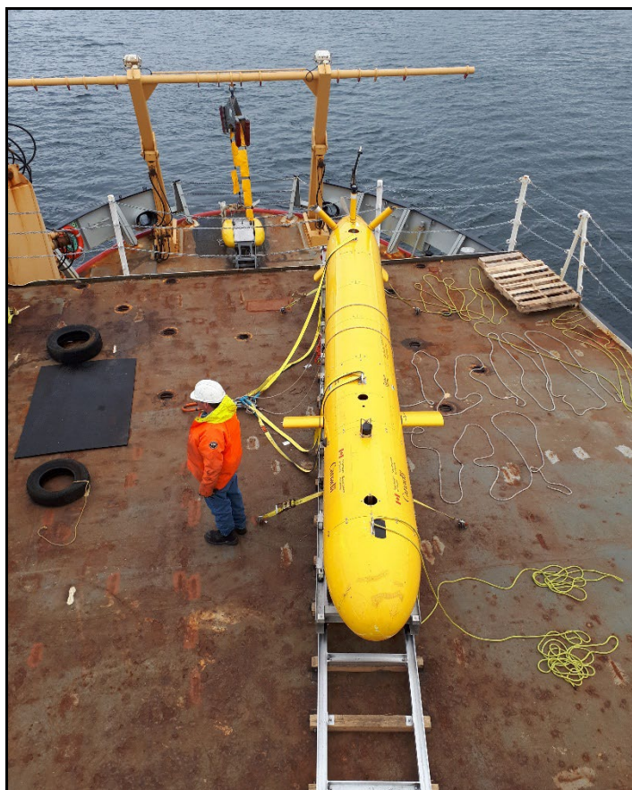
Figure 18- The AUV (ISE Eplorer 5000) on the flight deck on CCGS Hudson. Note the rail system for moving the AUV between the hangar and the flight deck.
