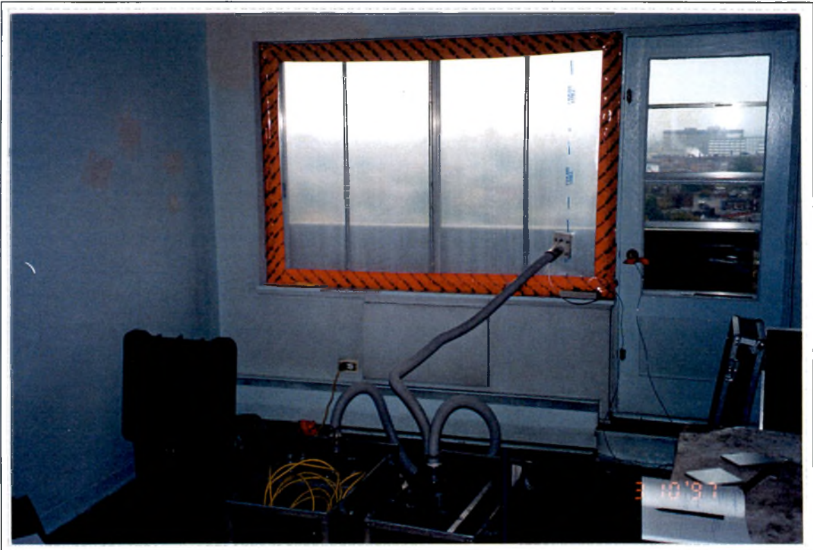
Photo #2: Typical setup for air infiltration measurements using the ASTM E-783 test method.
