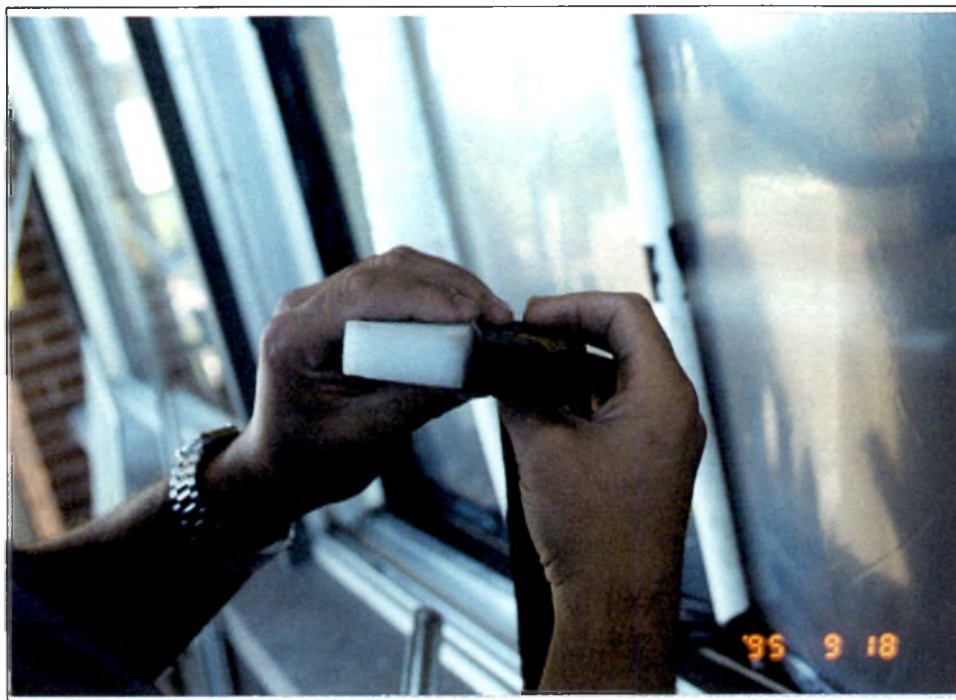
Photos #7: Comparison between a new pressure head sponge on the left, and the existing sponge from the MacDonald avenue apartments. The new foam provides for a much tighter seal at the window head and is wrapped to protect the foam from deterioration.
