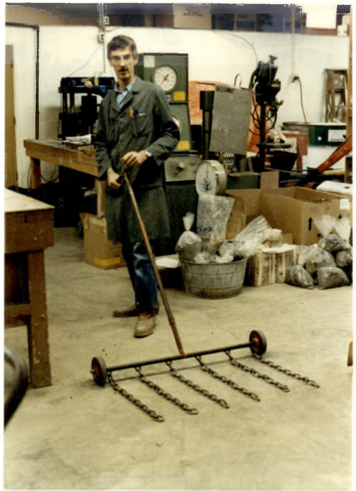
PHOTO B3: Typical chain drag device used to locate delaminations.
