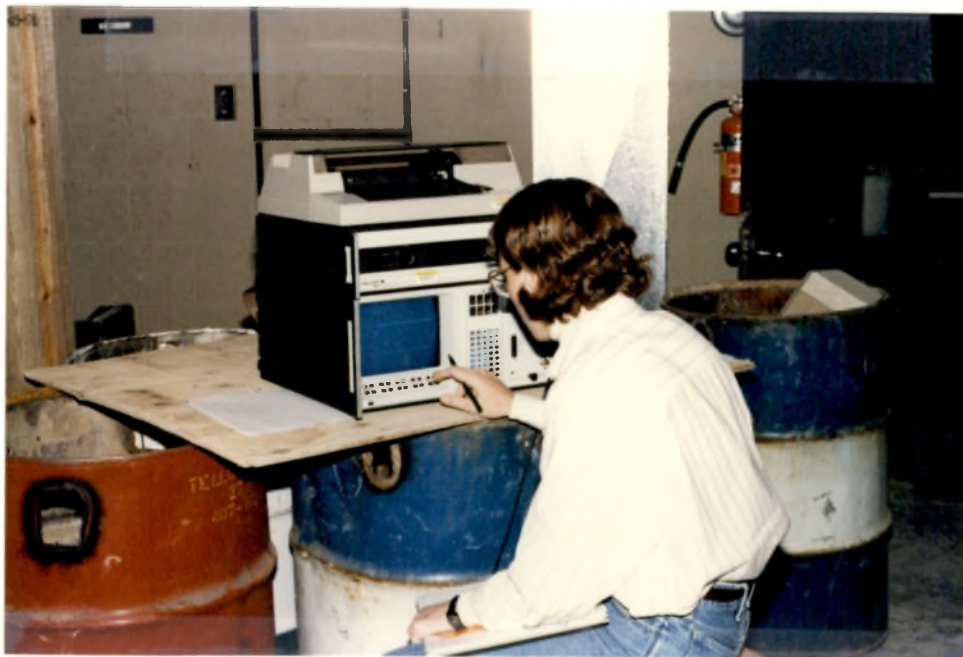
PHOTO B8: National Bureau of Standards data processing equipment. Storage oscilloscope, computer and disc drive at bottom, plotter on top.
