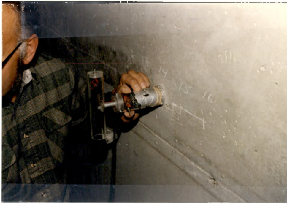
PHOTO B7: Point-contact receiving transducer used by National Bureau of Standards.
