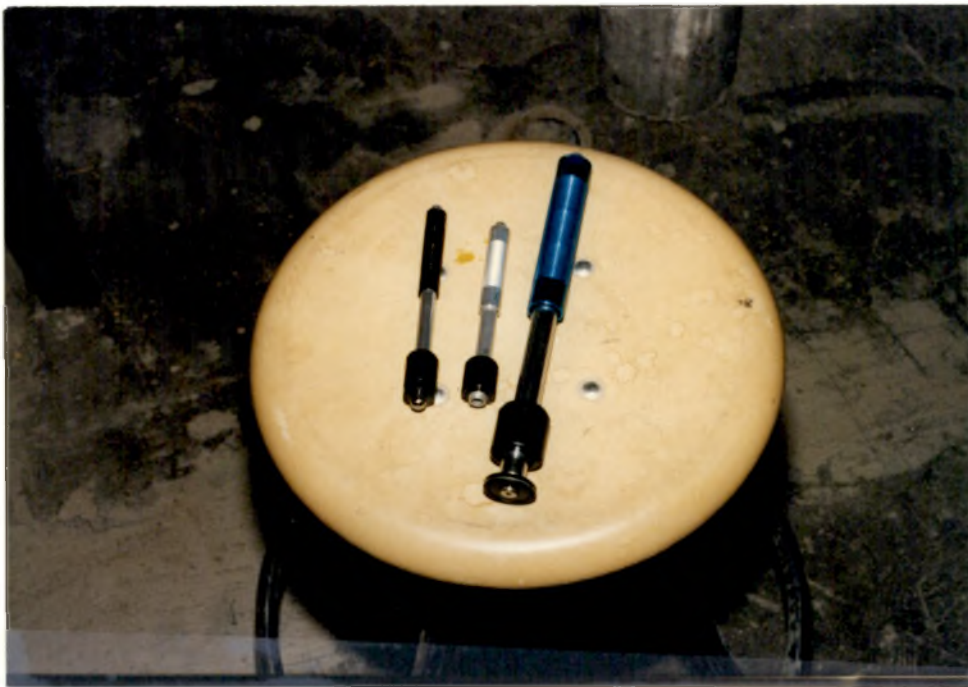
PHOTO B6: Impactors used by National Bureau of Standards to create the pulse.
