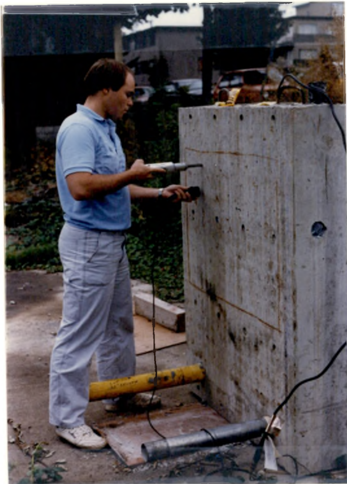
PHOTO B4: Impact-echo equipment in use. Transducer is in left hand, Schmidt hammer is used in right hand to create pulse.
