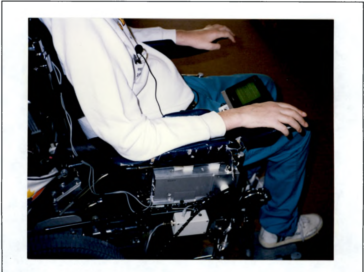
Figure 2 Wheelchair-mounted LCD Terminal and Communications Transmitter/Receiver.
