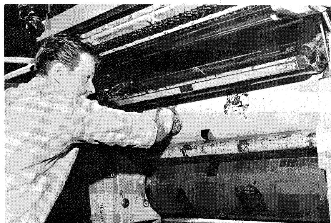
TURN AND TURN ABOUT — The image from the plate cylinder on the bottom has been transferred to the rubber-covered cylinder in the centre which, in turn, transfers it to the impression cylinder on the top that carries the paper.
