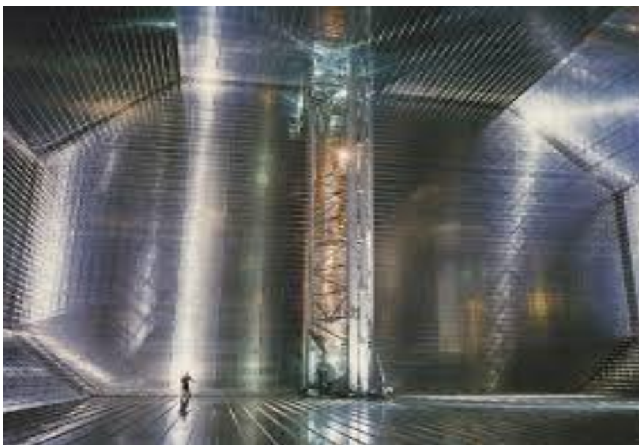
Inside the membrane tank of a typical 266,000 m 3 LNG carrier
