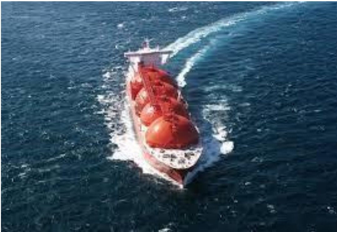
Typical 125,000 m 3 LNGC in Operation
