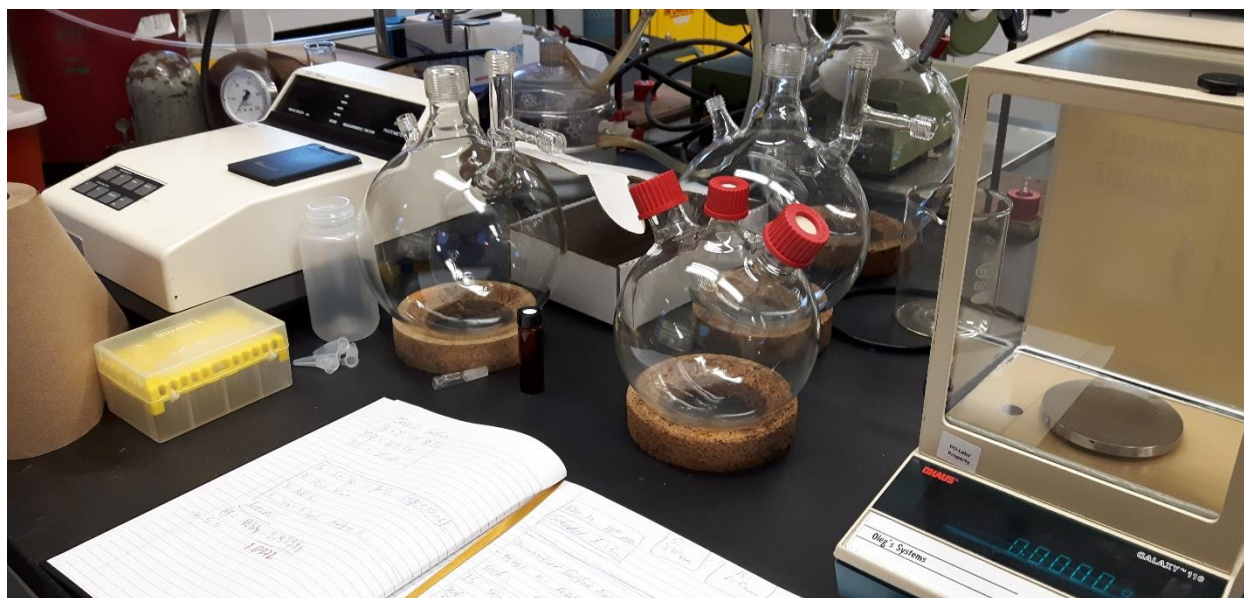
Figure 8. Spectrophotometer Pharmacia® LKB Novaspec II is on the left side of the photograph; analytical balances are on the right.
