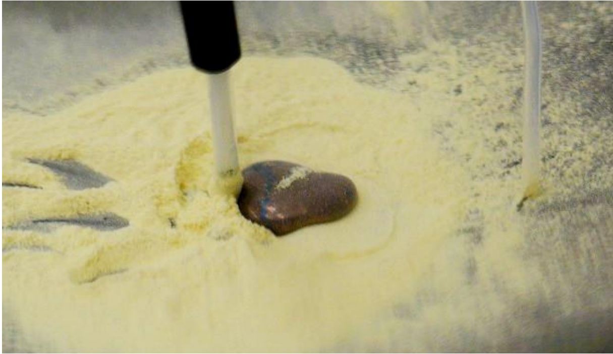
Figure 16. A photograph of the undisturbed mercury droplet, exposed to sulphur vapours.
