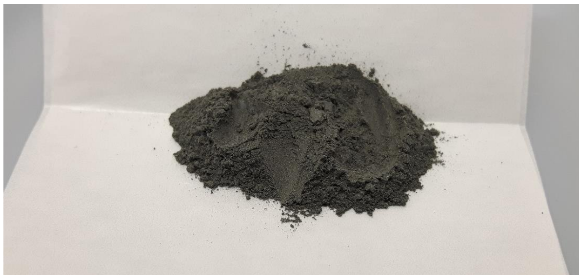
Figure 23. Mercury – sulphur mixture, reacted for five days, 150 rpm, 20 °C.
