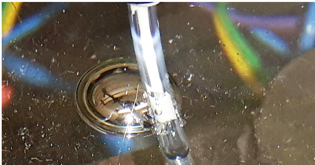
Figure 26. Mercury in vinegar. The temperature sensor placed in front of the mercury droplet.
