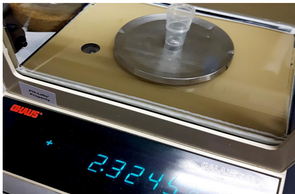
Figure 10. Gravimetric analysis. Mercury removed from the reactor is precisely weighted in a plastic container.
