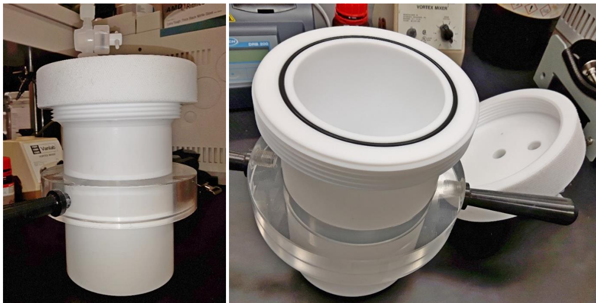
Figure 6. Two photographs of a reactor made of Teflon®.
