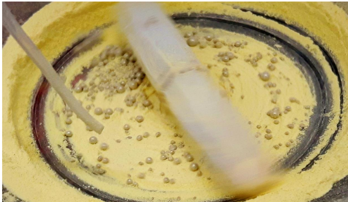
Figure 20. Mercury injected into reaction vessel with sulphur and mixed at 150 rpm.
