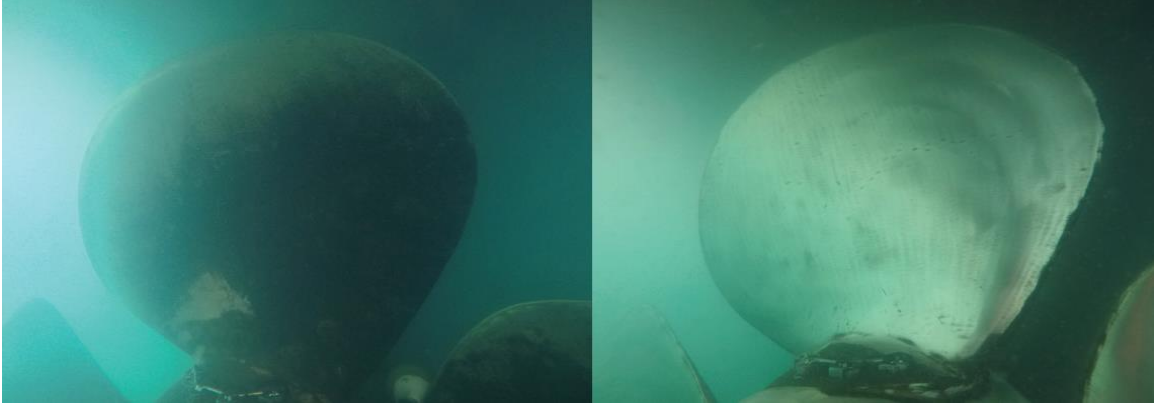
Figure 2. Typical propeller pressure face pre (left) and post (right) cleaning
