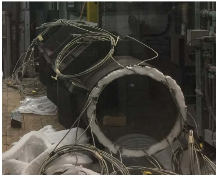
Figure 1 Calorimeter being instrumented with thermocouples on the outer shell and inner shell; and the hollow centre to be filled with insulation materials
