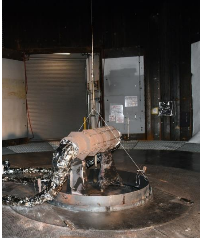
Figure 4-7: Suspended cable above calorimeter which held the plume thermocouples.
