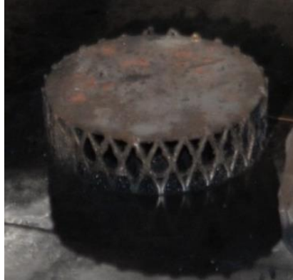
Figure 2-2: Diffuser for fuel introduction into the 2-m diameter pan.
