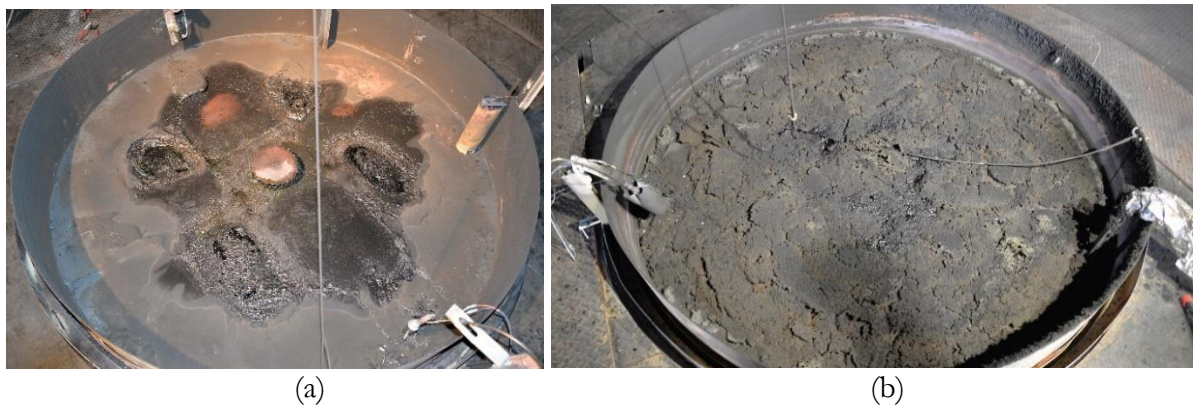
Figure 8-8: Post-test residue remaining from the (a) Bakken crude oil and (b) dilbit crude oil for non-continuous fuel feed tests.
