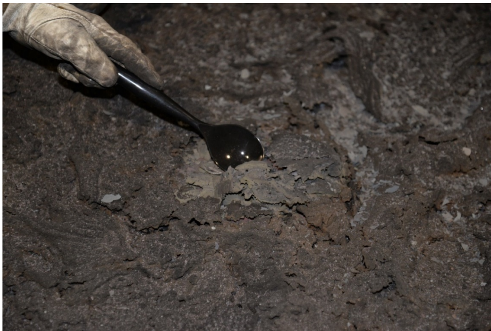
Figure 4-7. Close-up photo of sampling post-burn residue from the center of the pan for Test 3.1 on February 7.
