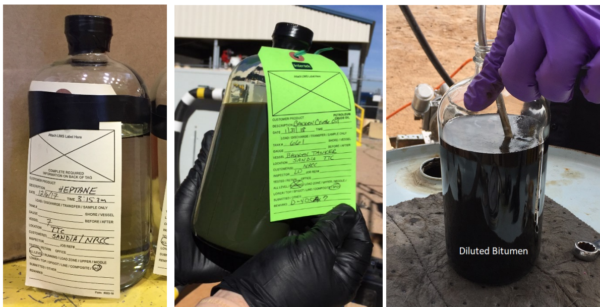
Figure 5-1. Comparison of heptane (left), Bakken (center) and diluted bitumen (right) visual properties captured during bottle sampling.
