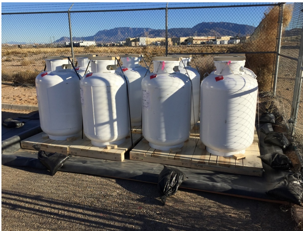
Figure 4-1. Photo of eight of the ten modified propane cylinders sent to Sandia to supply the dilbit pool fire testing.
