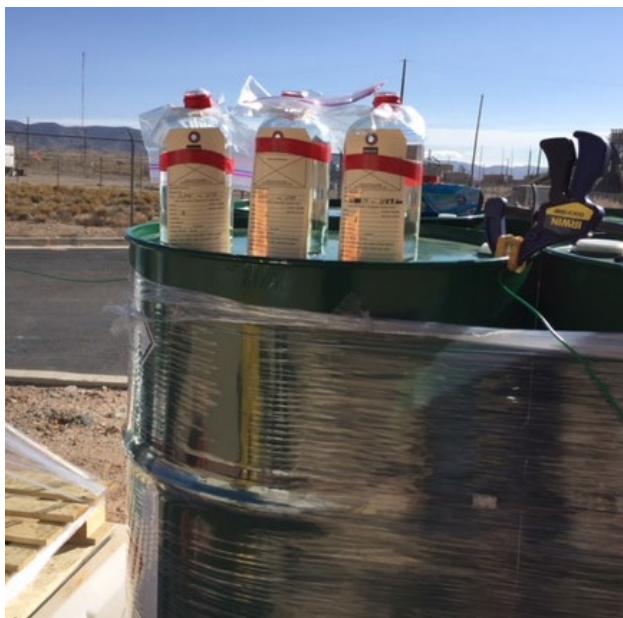
Figure 2-2. Photo of heptane source drum (green barrel) and sampling bottles (clear glass, three shown) used here.
