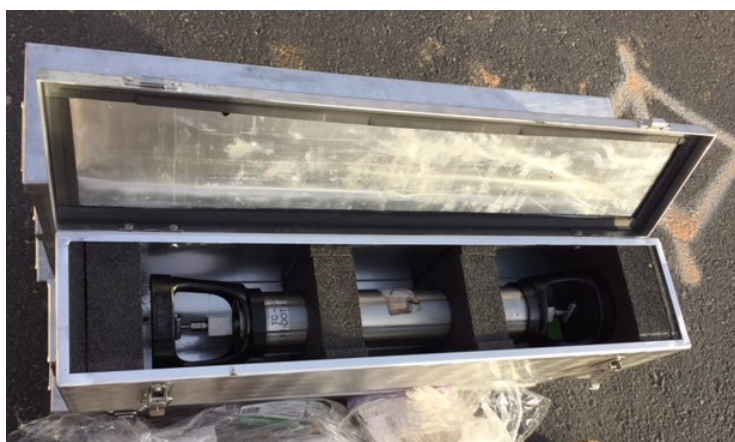
Figure 3-2. Photo of a 1-L capacity piston cylinder (in shipping case) used to collect pressurized crude oil during Sampling Event B4.
