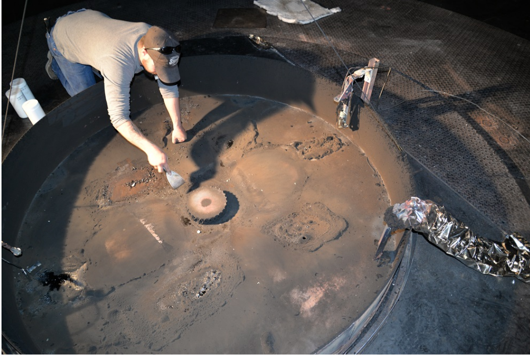
Figure 3-7. Photo of full pan taken after the January 31, 2018 pool fire (sampling event B7). Spot samples were collected and sent to an offsite laboratory for analysis.
