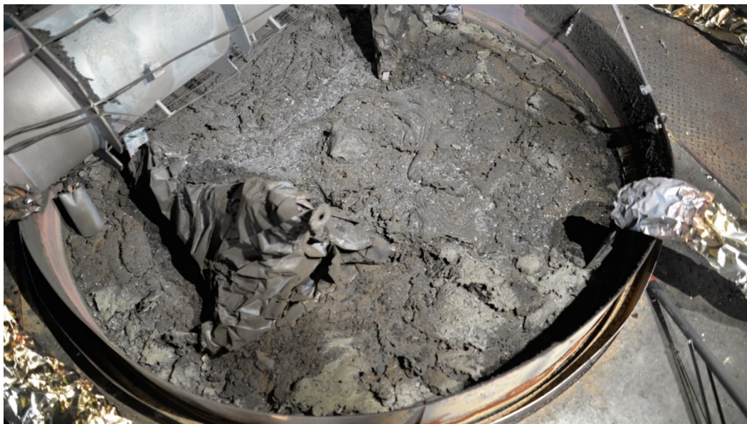
Figure 4-8. Photo of post-burn solids remaining after test 3.6. Total mass remaining was measured at 19.60 kg.
