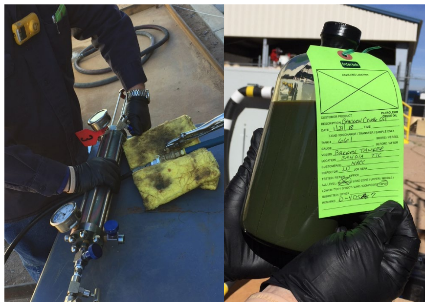
Figure 3-4. Photos taken during Sampling Event B6 (Burn Site Subsampling 3) at the Sandia thermal test complex on January 31, 2018, prior to the sixth and final 2-m pool fire. Left photo shows a 500-mL capacity floating piston cylinder during oil fill. Right photo shows a “Boston Round” glass bottle containing about 700 mL Bakken crude.
