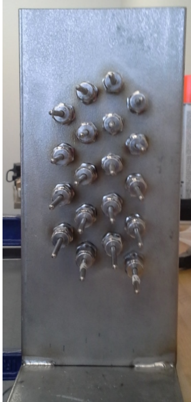
Figure 1. Thermocouple rake for measuring temperatures in the fuel and substrate.
