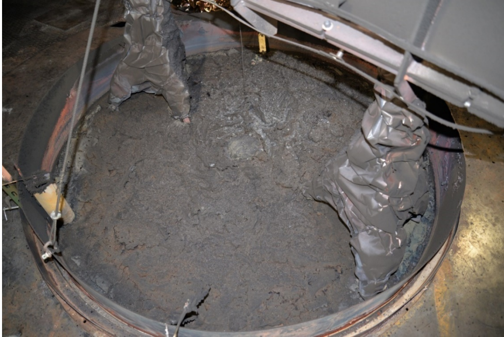
Figure 4-6. Photo of post-burn solids remaining after Test 3.1. Total mass of solids was measured at 31.48 kg.
