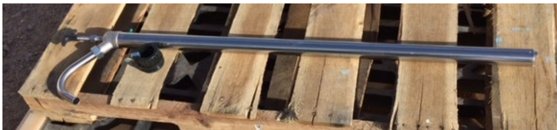
Figure 2-1. Photo of the manual drum pump (drum thief sampler) used to transfer heptane from the drums to the glass bottles.
