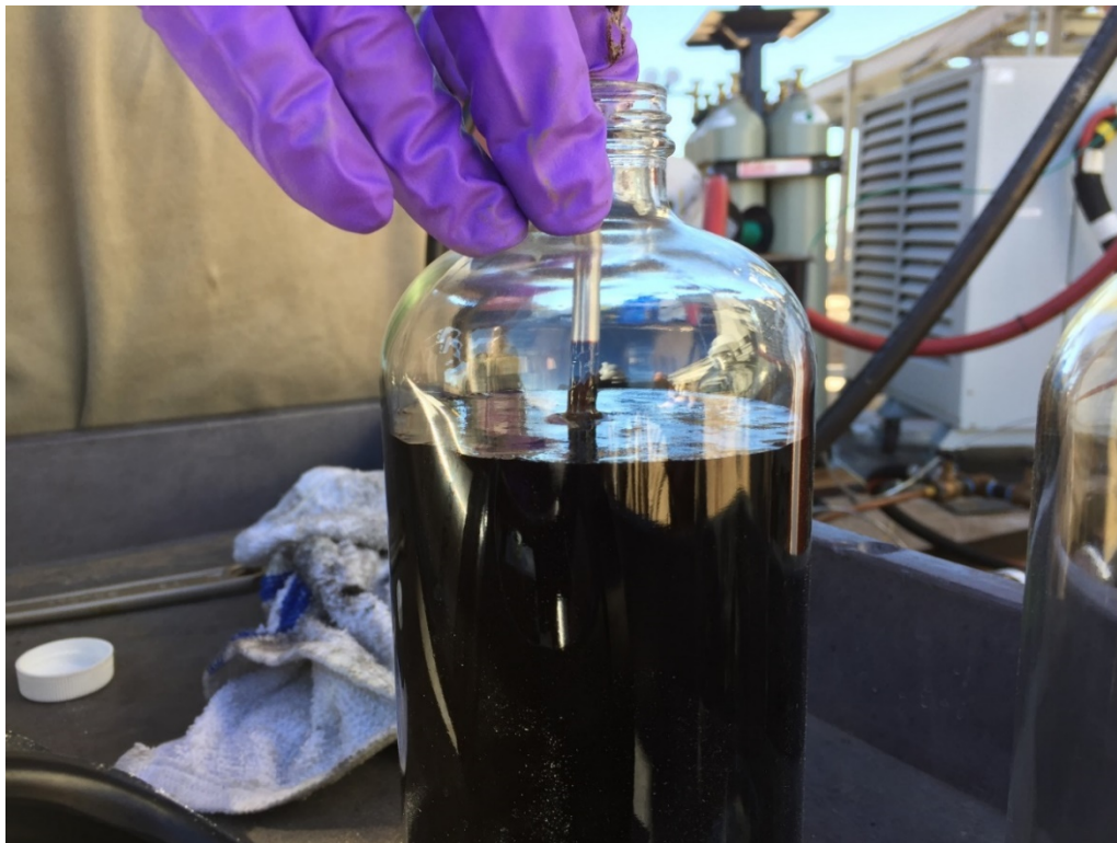
Figure 4-4. Photo of unpressurized glass bottle during ASTM D4057 fill process with dilbit from Tank 12.
