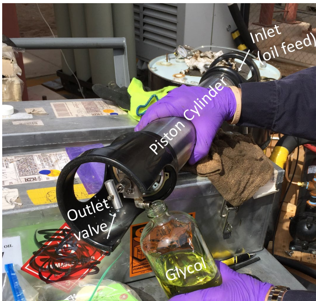
Figure 4-5. Photo of pressurized piston cylinder fill process with dilbit from Tank 9. Oil feed on the far end of the cylinder moves the internal piston while displacing glycol through the outlet valve from the close end. The volume of glycol displaced is a primary indicator of sample volume captured in the cylinder.
