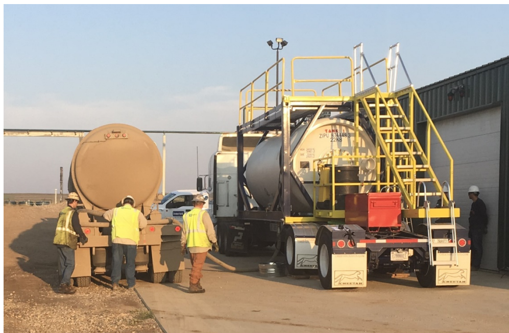
Figure 3-1. Sandia custom pressurized oil tanker (right) taking a load of crude while displacing water to vacuum truck (left)
