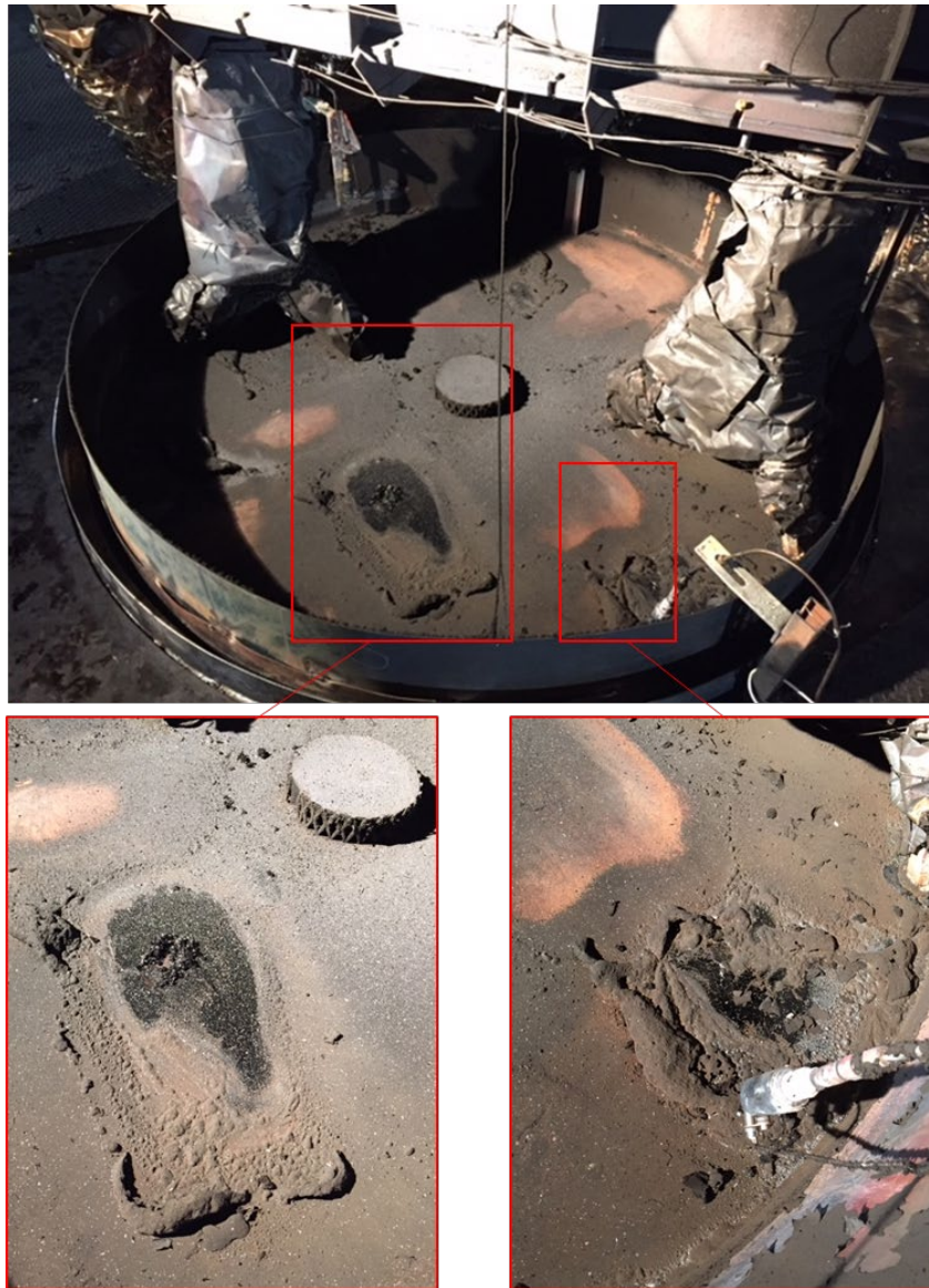
Figure 3-6. Photos of full pan with two insets taken after the January 19, 2018 pool fire, sampling event B5. Spot samples were taken and sent to an offsite laboratory for analysis.
