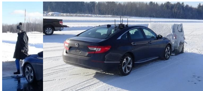
Figure 14. Advanced driver assistance systems testing in winter conditions. Images of cars with advanced driver assistance systems tested under snowy conditions, responding to pedestrians and other vehicles.
