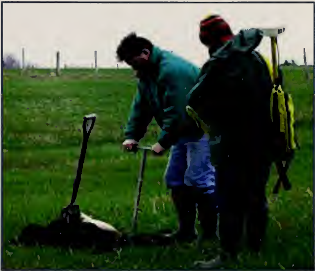
Sampling to classify soil profiles in the Bras d'Henri Watershed
