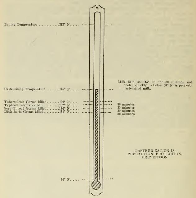
carrying out home pasteurization of the daily milk supply. The method as outlined employs the same temperatures and time as used in large commercial dairies, and where carefully followed will give efficient pasteurization.
