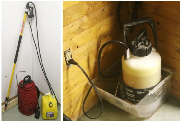
Figure 38. De-icing equipment available at Fond-du-Lac Airport: West Wind's equipment on left, another operator's equipment on right (Source: TSB)
