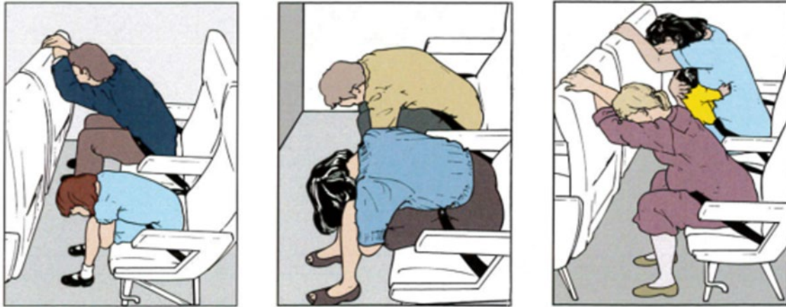
Figure 23. ATR 42 recommended brace position, as illustrated on the safety-features card (Source: West Wind Aviation L.P.)
