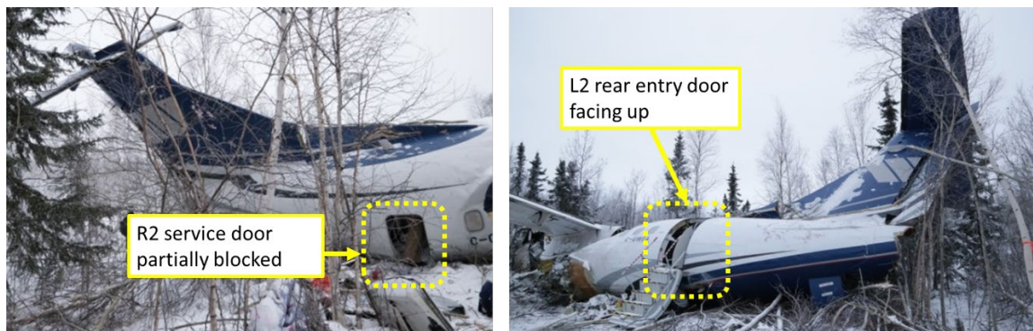
Figure 29. Orientation of the service door (R2) (left image) and the rear entry door (L2) (right image) (Source: TSB)
