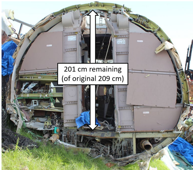
Figure 12. Cross-sectional view of the forward fuselage, just aft of the cockpit, looking forward, from later off-site examination (Source: TSB)
