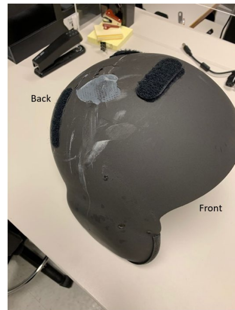
Figure 7. Impact marks on top of the pilot's helmet (Source: SAG, with TSB annotations)
