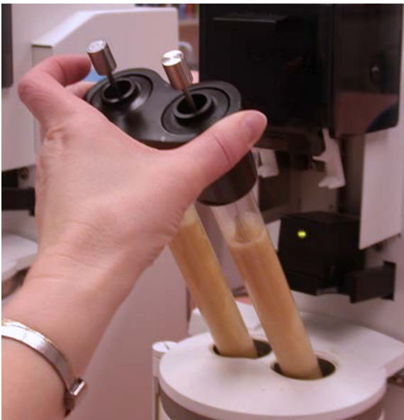
Figure 3 Running monthly Falling Number check test sample.
