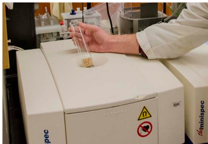
Figure 1 Pulse nuclear magnetic resonance (NMR) instrument used to analyse crude oil content.
