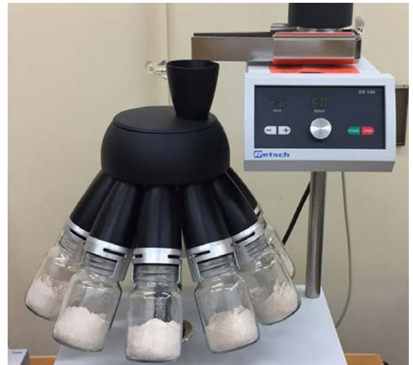
Figure 2 Front view of rotary divider; representatively dividing samples for the falling number check test.
