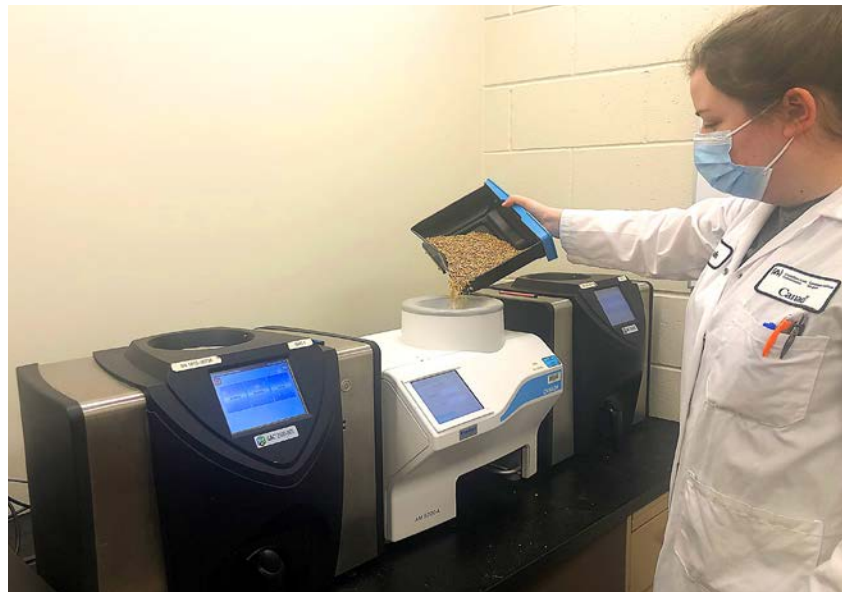
Figure 4 Moisture meters used for analysis of the moisture check test sample: AM522 Perkin Elmer and GAC Dickie John.
