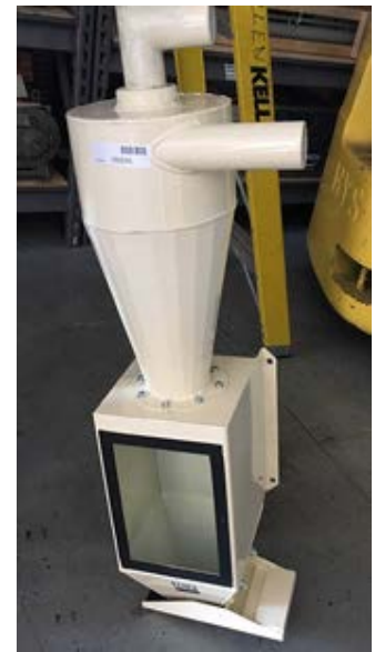
Figure 16: Sample collector using a vacuum pump with a cyclone
