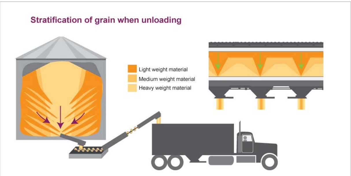
Figure 2: Stratification of grain when unloading
