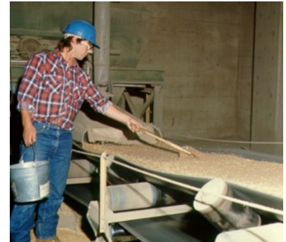
Figure 32: Sampling grain from a horizontal belt
