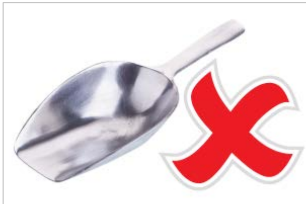
Sample size can be variable if using this type of scoop, therefore it's unsuitable for obtaining a consistent sample size.
