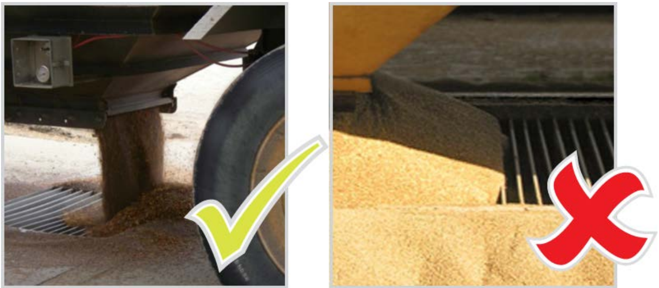
Figure 29: Manual stream sampling over an open pit
