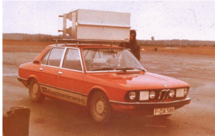
Figure 16: 10 GHz automotive radar system built by VDO, early 1970's [95].
