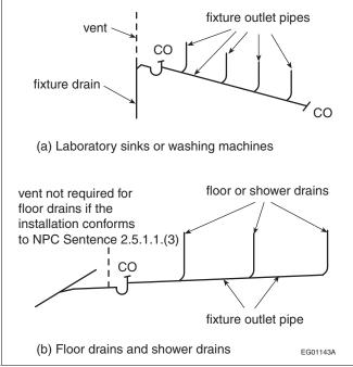
Figure A-2.4.5.1.(3) Single Traps for Fixture Groups
