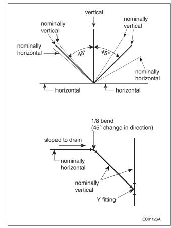
Figure A-1.4.1.2.(1)-J Nominally Horizontal and Nominally Vertical
