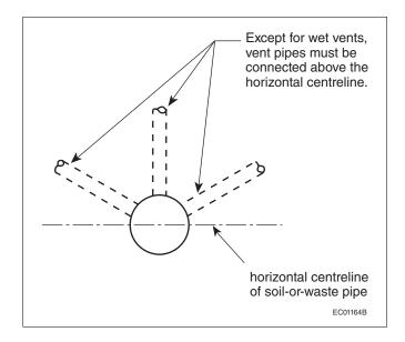
Figure A-2.5.6.2.(2) Vent Pipe Connections
