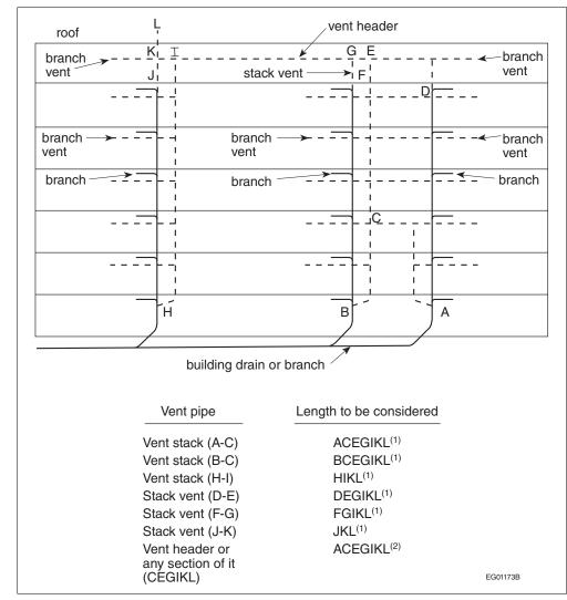
Figure A-2.5.8.3. and 2.5.8.4.-B Lengths to be Considered When Sizing Vent Pipes Notes to Figure A-2.5.8.3. and 2.5.8.4.-B: (1) See Sentence 2.5.8.4.(2).
