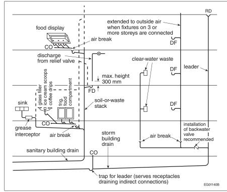
Figure A-2.4.2.1.(1)(a)(ii) and (e)(vi) Indirect Connections
