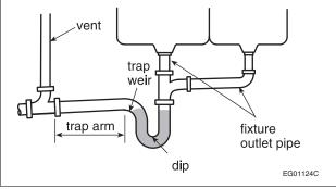
Figure A-1.4.1.2.(1)-H Fixture Outlet Pipe and Trap Arm
