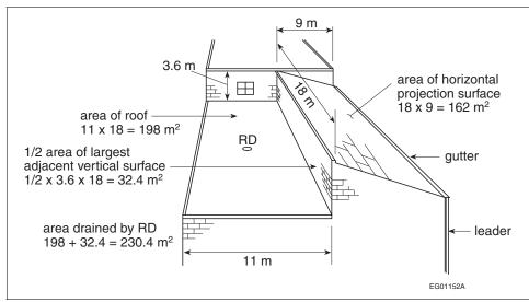
Figure A-2.4.10.-B Storm Drainage Areas (Example 1)
