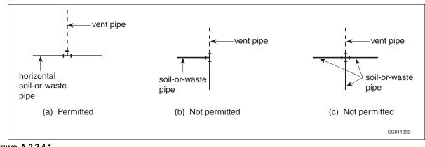
Figure A-2.2.4.1. T Fittings in Drainage Systems
