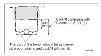
Figure A-2.3.5.1.(1)(a) Backfilling of Pipe Trench
