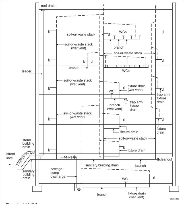
Figure A-1.4.1.2.(1)-F Drainage System
