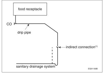
Figure A-2.4.7.1.(9) Cleanouts for Food Receptacle Drip Pipes Note to Figure A-2.4.7.1.(9): (1) See Article 2.4.2.1.
