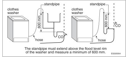
Figure A-2.4.9.3.(3) Standpipe Installation for Clothes Washers
