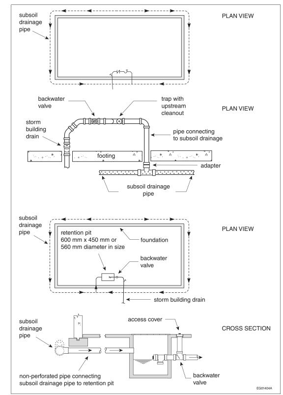
Figure A-2.4.5.3.(1) Subsoil Drainage Connections
