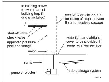
Figure A-2.4.6.3. Arrangement of Piping at Sump
