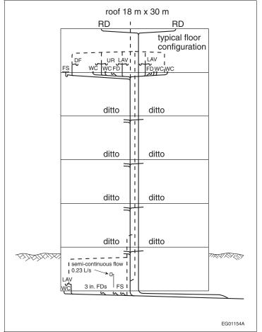
Figure A-2.4.10.-D Building Drainage System (Example 2)
