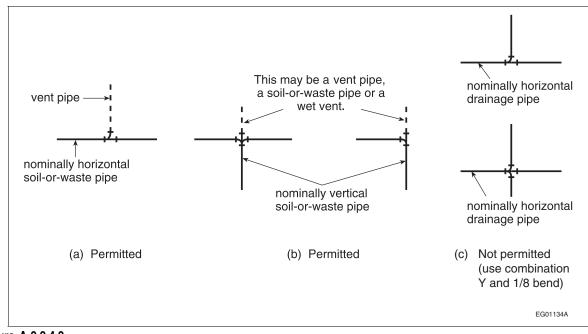
Figure A-2.2.4.2. Sanitary T Fittings in Drainage Systems
