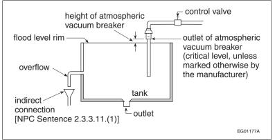
Figure A-2.6.2.10.(2) Installation of Atmospheric Vacuum Breakers
