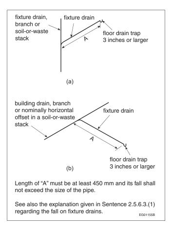
Figure A-2.5.1.1.(3) Trapping of Floor Drains
