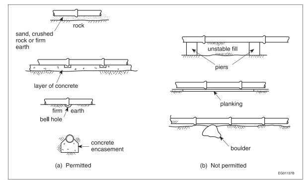
Figure A-2.3.4.6.(1) Support for Underground Piping
