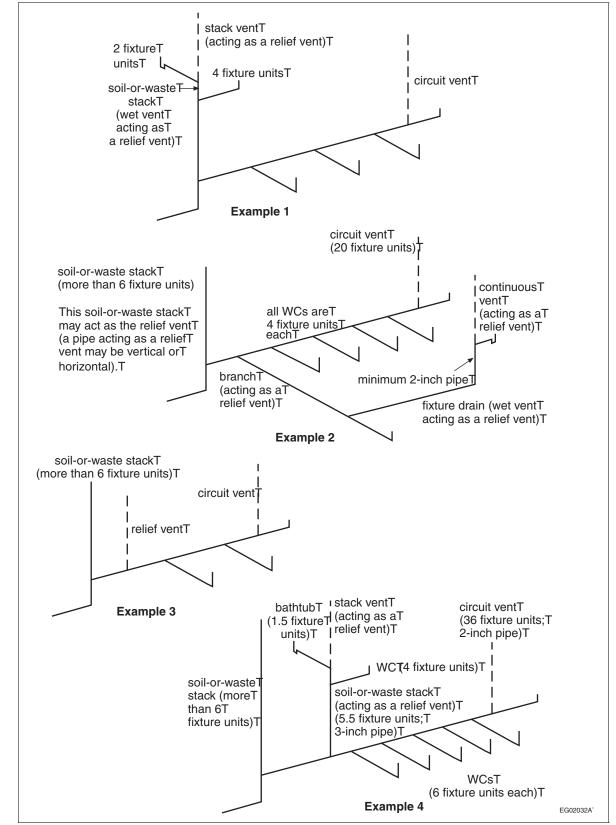
Figure A-2.5.3.1.-E Example of Circuit Venting Described in Sentence 2.5.3.1.(4)
