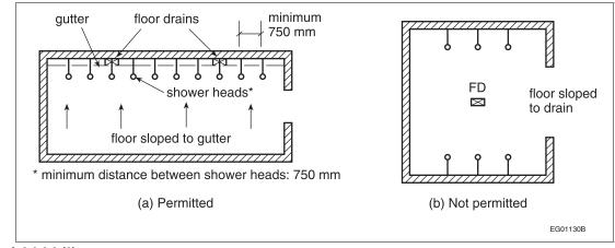
Figure A-2.2.3.(3) Shower Drainage (Plan View)
