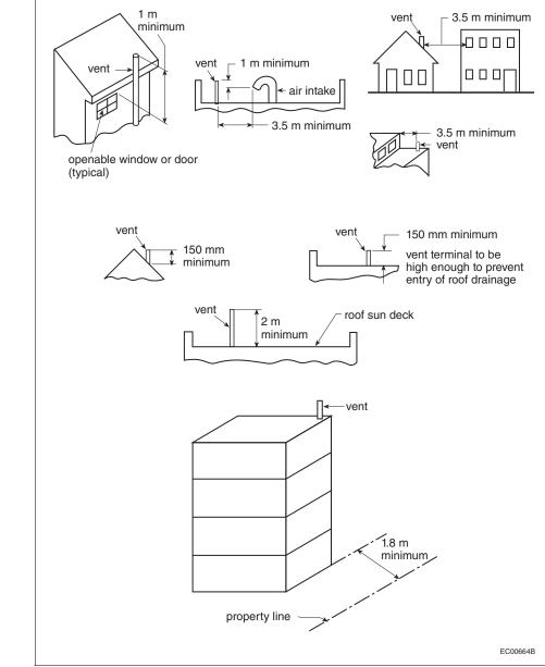
**A-2.5.6.5.(4) Vent Terminals.** No vent pipe other than a fresh air inlet may terminate within the limits indicated.
