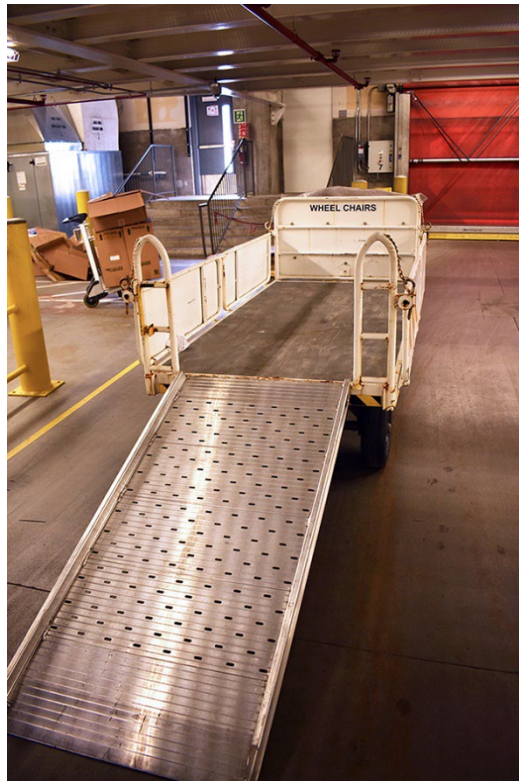
Figure 4. Repurposed luggage cart to assist in handling powered mobility aids
