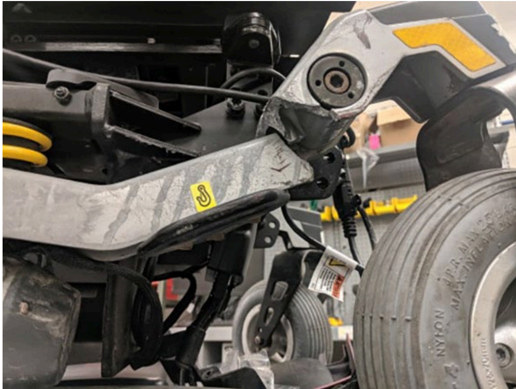
Figure 14. Photo of a mobility aid, damaged beyond repair due to a cracked frame (note securement point sticker)
