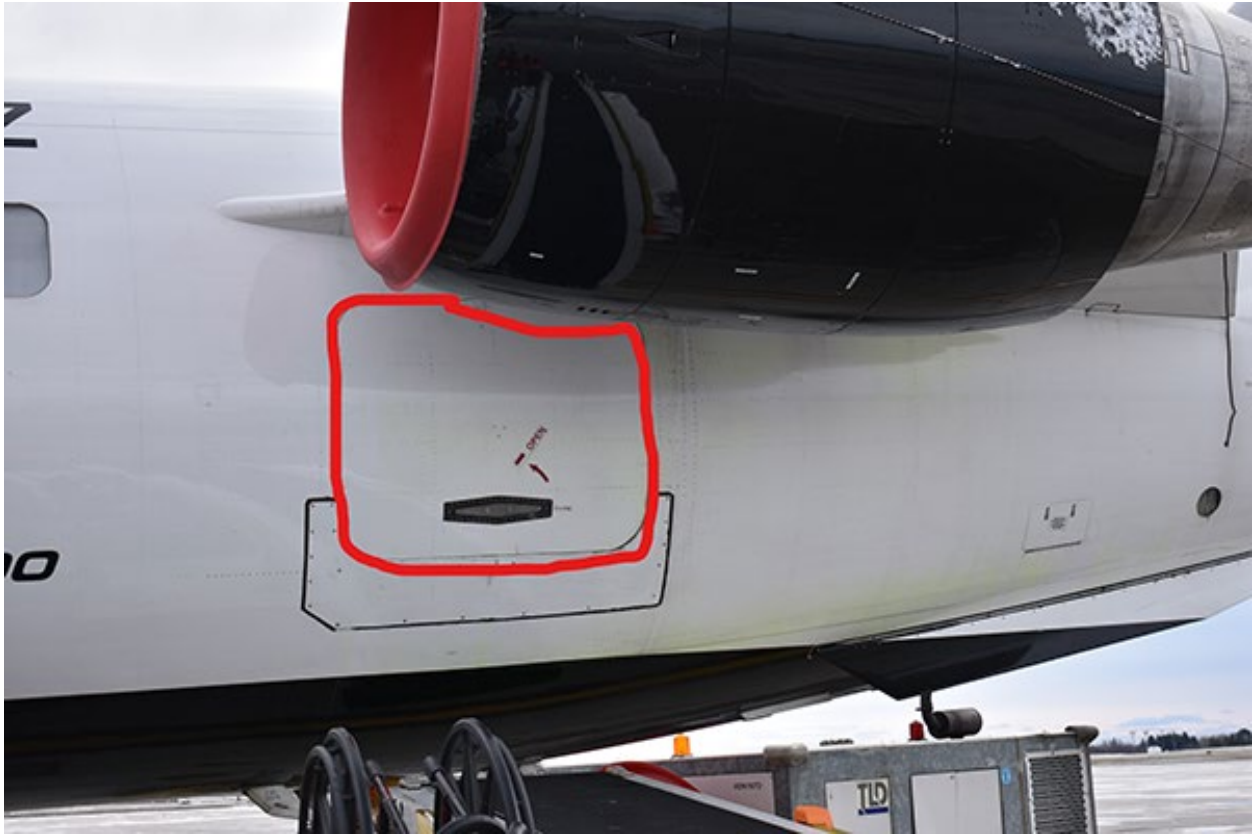
Figure 5. Example of a cargo door, with the engine slightly blocking access to full cargo door dimension, as shown in red outline
