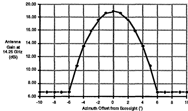
Fig. 3. Mobile Terminal Transmit Antenna Gain (Azimuth Cut)
