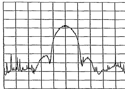
Fig. 11 BPSK signal spectrum at modulator output
