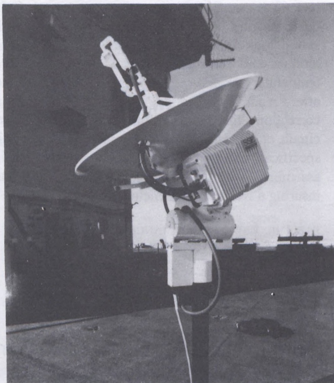
Figure 8. Ku-Band Integrated Radio mounted on servo-stabilized 0.8m antenna platform.
