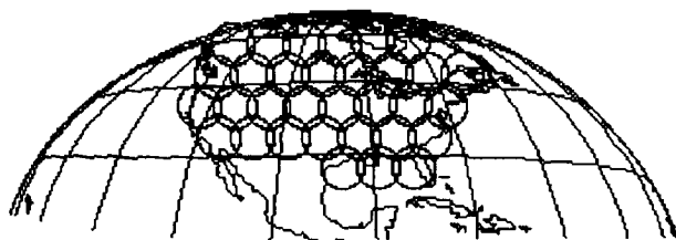
Fig.2 32 beams North America coverage which support personal satellite communications at 2.01GHz Beam diameter is 629km \phi at nadir.
