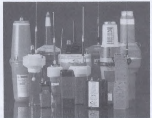
Figure 9: Various models of 406 MHz distress beacons
