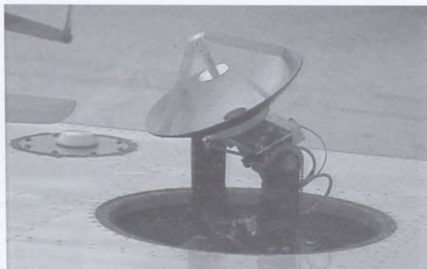
Fig. 3 - Picture of the aircraft mounted Cassegrain antenna and the GPS antenna
