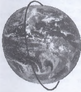
Figure 3: Orbital plane of a polar-orbiting satellite
