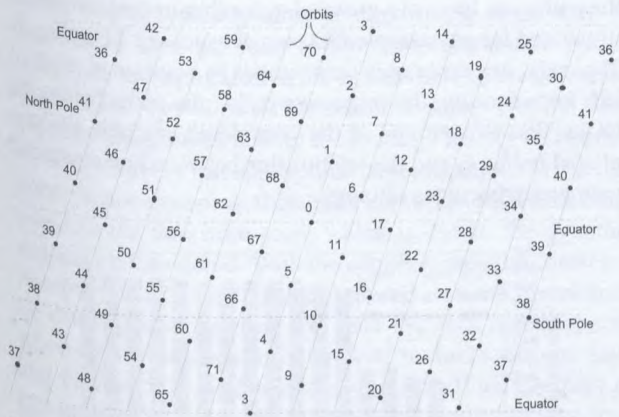
Fig. 1. Planar projection of the M-Star constellation at t = 0 . Distances and angles are not true to scale.
