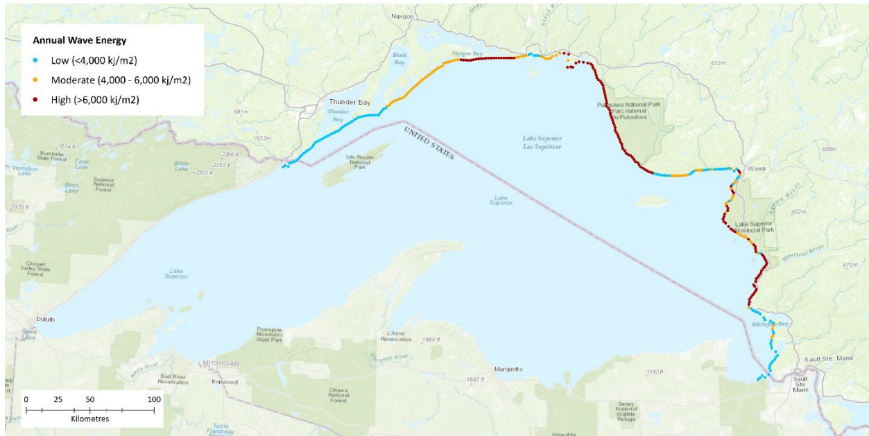
Figure 3. Results of the wave energy density analysis on Lake Superior. Wave energy density was not modelled in bays or connecting channels
