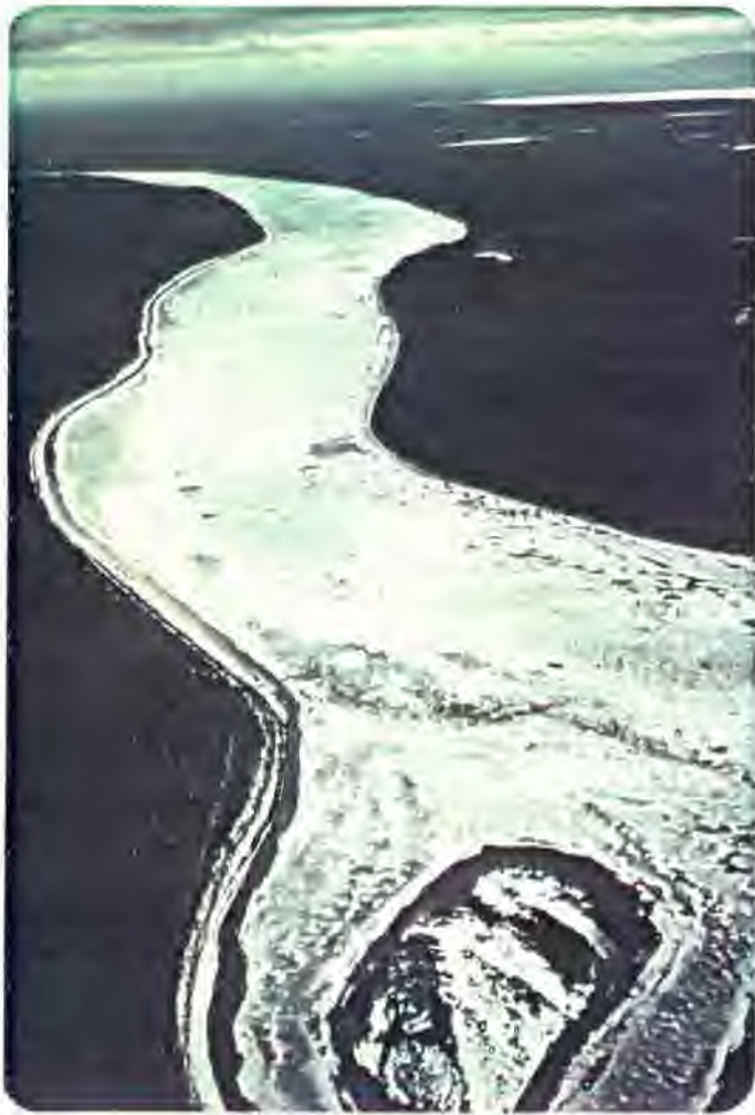
PHOTOGRAPH 1. Liard River viewed upstream from LKP 21, May 7, 1982, 1540 MST, showing pre-break-up ice conditions. Note the deteriorating but continuous ice cover, shore leads, and bottomfast ice along right bank.
