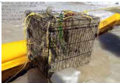
BASKETS FILLED WITH OIL SNARE INSPECTED DAILY TO DETECT THE PRESENCE OF SUBSURFACE OIL
