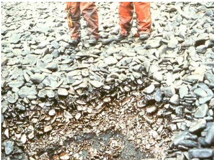
Figure 7.9 Cobble beach on which emulsified oil has penetrated > 1 m before reaching an impermeable hard sand layer
