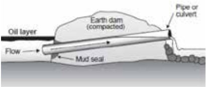
CHANNEL BARRIER – UNDERFLOW DAM
