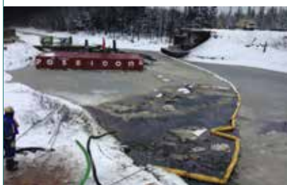
BUBBLING SYSTEM USED TO OPEN AND MAINTAIN ICE FREE AREA FOR OIL RECOVERY
