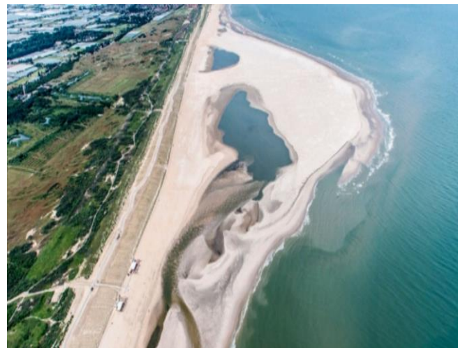
Figure 20. Mega-sand nourishment at the Delfland Coast, Netherlands.
