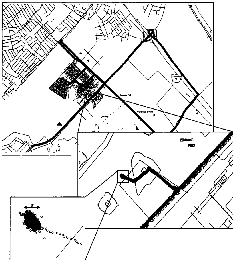
Figure 7. GPS Determined Locations of the TAGA Bus During Sampling Runs (at Different Levels of Resolution).
